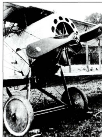
This view shows off the 160 hp twin-row Oberursel motor of Boelcke’s D III 352/16 on the Jasta 2 aerodrome. After Boelcke’s death, this aircraft was presented to the Prussian military museum in Berlin for preservation. It was returned to the Fokker factory to be refurbished, and its finish was considerably altered for its museum exhibition. The DIII was destroyed in World War 2
