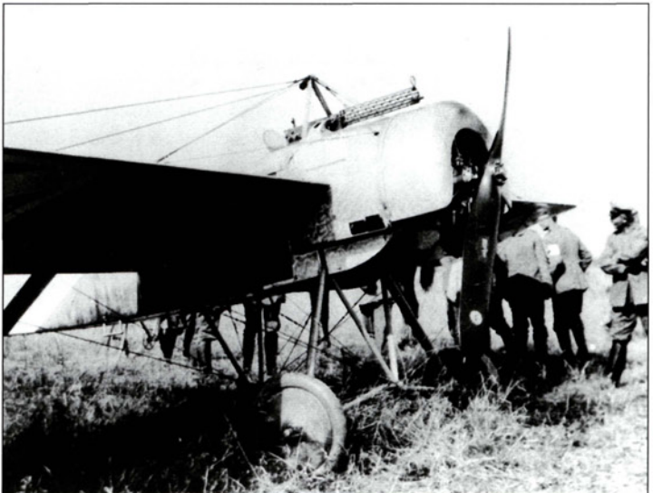
A less familiar view of Immelmann's E 1 reveals the LMG 08 machine gun. The cowling was fitted with a blast plate below the muzzle of the gun for protection from blast debris, and the staining seen there proves the weapon has seen use. Note the opaque appearance of the fabric, even in strong sunlight. The propeller displays the trademark of the Garuda firm
