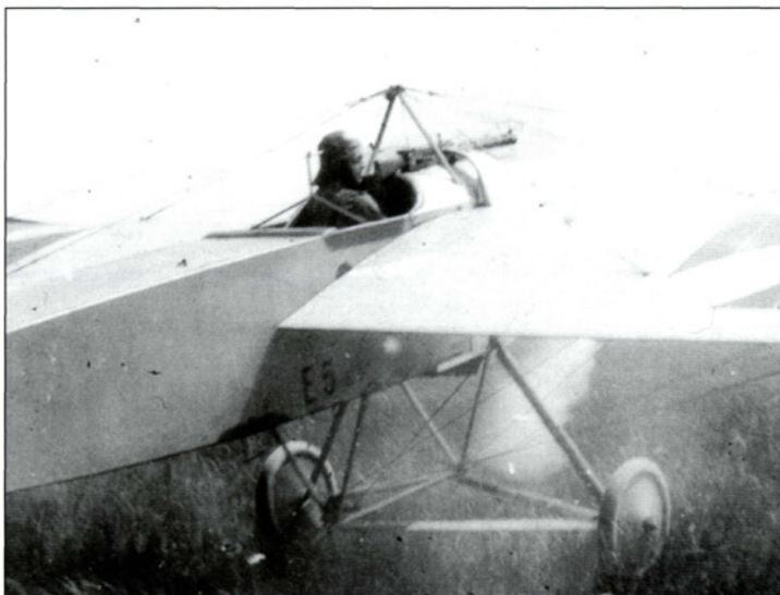
Kurt Wintgens is seen running up the 80 hp Oberursel of his E I 5/15 almost certainly whilst serving with Bavarian FFA 6 in July 1915. This aircraft retains the high shoulder-mounted wing and a Parabellum gun, and had a headrest to steady the pilot's head while aiming. It seems highly likely that Wintgens used this aircraft to obtain an unconfirmed victory over a French Morane on 1 July 1915
