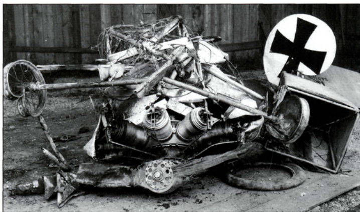
The tangled wreckage of Fokker E III 246/16 was collected for evaluation and study in an attempt to determine the true cause of Immelmann's death. The one remaining arm of the propeller appears neatly severed in line with the machine gun barrel, providing support for the view that faulty synchronisation had caused the crash. The aft portion of the fuselage had broken away and remained nearly intact, and the Wk-Nr 545 was stencilled neatly on the elevator
