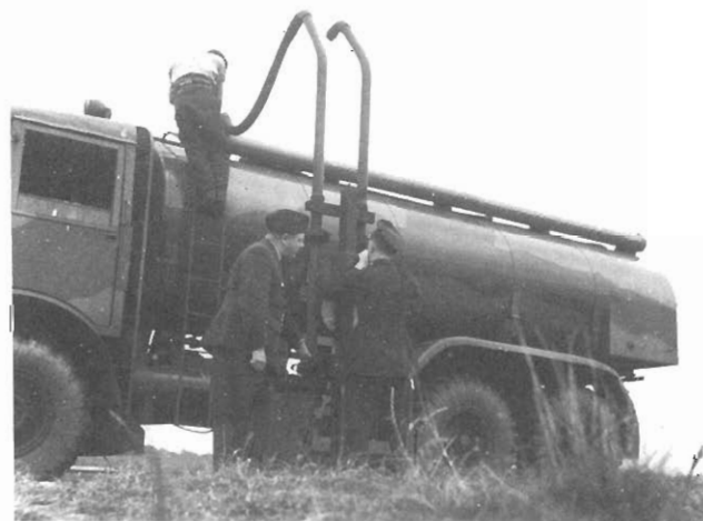
13 Petrol supplies being delivered into an airfield's main storage tanks from a delivery tanker. At left, the equipment officer, whose responsibilities included checking the quantities delivered. (Imperial War Museum)
