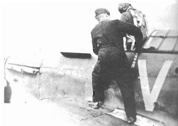
18 Lewis is helped into the cockpit of VY-R; the port shoulder strap of the Sutton harness is under the mechanic's right hand. The protruding plate forward of the cockpit was to shield the glare from the exhausts during night flying. (Life Magazine via R. L. Ward)
