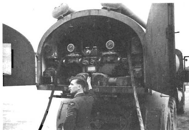
15 Checking the controls on an Albion 350 Bowser as fuel is pumped into an aircraft. (Imperial War Museum)
