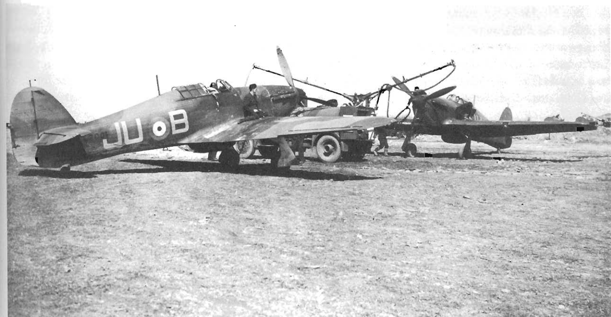
14 Hurricanes of No.111 Sqn. refuelling from an Albion 350 Bowser at Wick, February 1940; at this time the squadron's role was to give air cover for shipping entering
