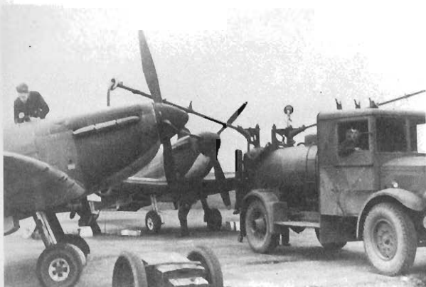
7 Spitfire Mk I or II fighters being refuelled, early 1940. Background aircraft has port underside painted black and individual letter 'O' painted below the spinner. (via R. L. Ward)
