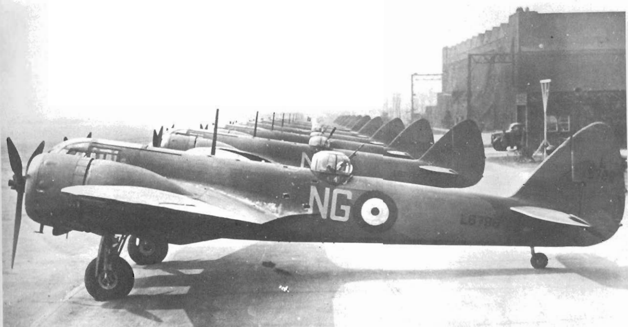
5 Blenheim Mk 1Es of No.604 Sqn., Aux AF; Northolt, 6 April 1940. Note gun-pack under fuselage of nearest
