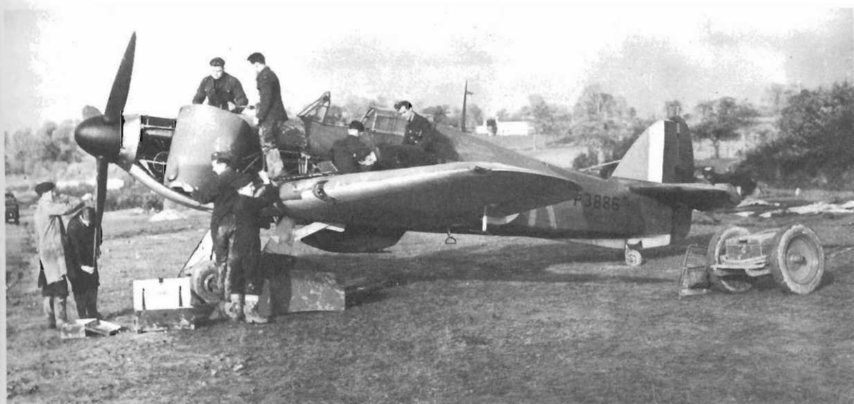
12 Tangmere, 1940; Hurricane Mk. I, P3886, UF-K of No.601 (County of London) Sqn., Aux AF, undergoing servicing. Note the dress of the groundcrew, ranging from denims to service dress – the coat-type overall is of interest. Note also 'trolley acc' near the tail – the normal type of
