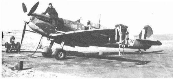
38 Roy Briggs of No.131 Sqn. with his Spitfire Mk. Vb, NX-Z 'Karmie', in early 1942. The aircraft is plugged into its starter, and the pilot's parachute rests on the wing-tip. (via R. L. Ward)
