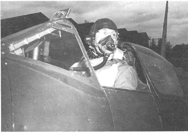
24 Spitfire pilot wearing later issue flying helmet (note angular earphone housings) and oxygen mask. The seat is in the raised position used for take-off, and would be lowered to allow the canopy to be closed once the fighter was airborne. (Imperial War Museum)
