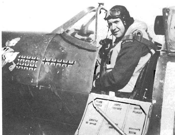
32 Flt. Lt. J. A. Gibson, a New Zealand pilot of No.457 Squ., in the cockpit of his Spitfire Vb, BL351, BP-H at Jurby in December 1941. Note the crowbar – for use of the pilot if breaking his way out of a crashed aircraft – held in clips inside the cockpit access panel. The right hand victory cross in the top row is halved, possibly indicating a shared victory. (Frank Smith via R. L. Ward)
