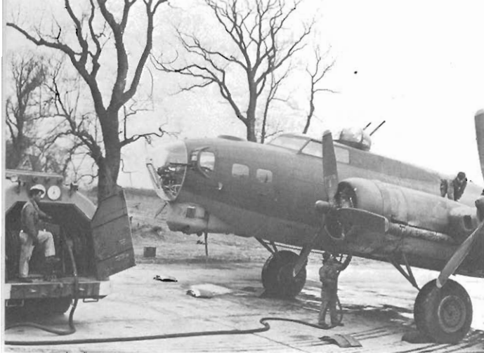
24. Part of the 100-octane fuel load being pumped into the inboard tanks of 42-21313, a B-17G of the 91st BG, at Bassingbourn on 10 February 1944. The B-17G could take 2,810 US gallons in its built-in tanks, and 3,630 maximum with bomb-bay tanks. The ship illustrated here is a Vega-built Fortress with short perspex nose cone.
