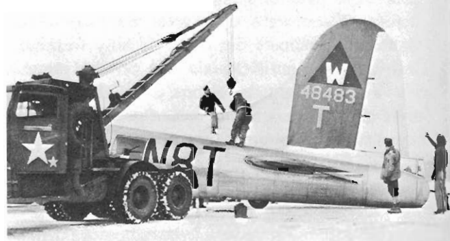
38. With an airfield crane providing mechanical muscle, ground crewmen prepare to lift B-17G 44-8483, N8-T of the 600th BS, 398th BG off its ass after a tailwheel collapse on landing at Nuthampstead, Herts., during winter 1944-45. Note yellow serial and ID letter on the red fin strip of the 1st Wing, 1st Division.
