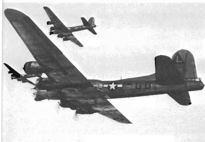
31. The basic three-ship combat element of the 8th Air Force demonstrated by two B-17Gs from the 381st BG's 532nd BS (top) and one (foreground) from the 534th BS. Note fully retracted H2X housing on the nearest machine.
