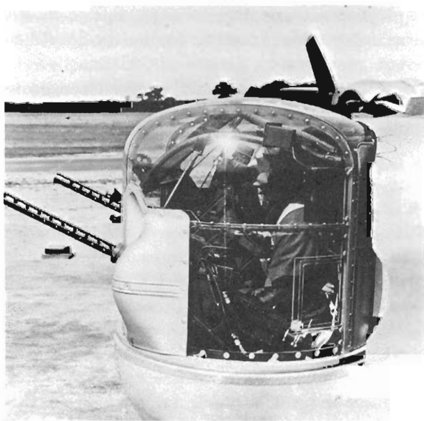
35. Meanwhile, up front . . . S/Sgt. Edward J. Mickey in the Emerson nose turret of a B-24. Nose turret armament was an important factor in cutting losses from the head-on attacks which claimed so many.
