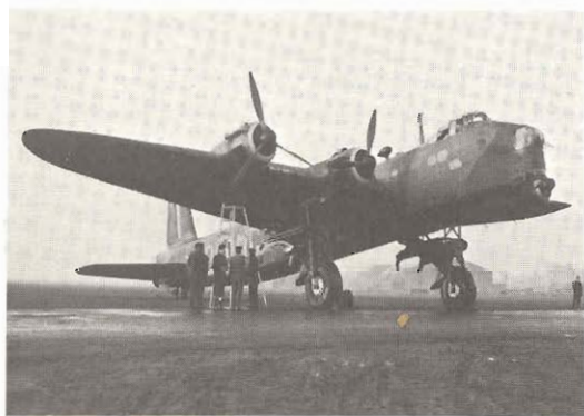
30. The first of the 'heavies' – Short Stirling MG-D of No. 7 Sqn, which received the type in August 1940. Note the enormous ground clearance, and the ladders needed to service the engines.
