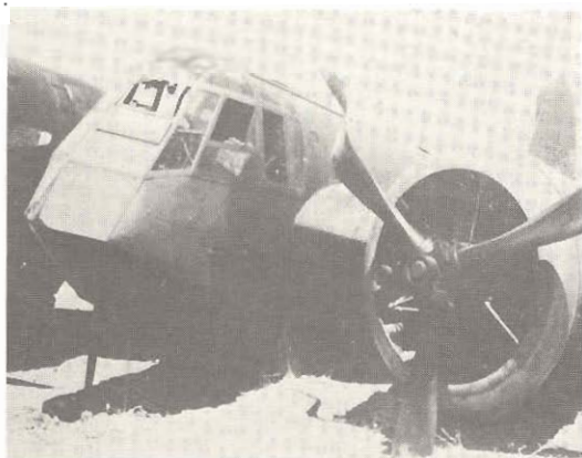
9, 10. The result of a port undercarriage collapse suffered by Blenheim Mk I, L8500. (via R. L. Ward)
