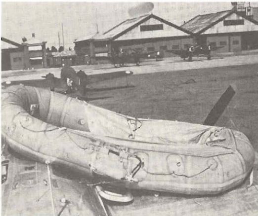
27. This seven-man dinghy was stowed in the wings of bomber aircraft and released on impact with water. This typical example was in fact photographed at one of the E.A.T.S. schools in Australia. (via R. L. Ward)
