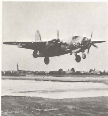
31. The 'shark-mouth' identifies this aircraft as belonging to the 44th BS, 320th BG as it lands at Dijon/Longvic, France. The radio call number 2107541 identifies it as a B-26C-45-MO Marauder built by Martin at Omaha, Nebraska. (USAF)
