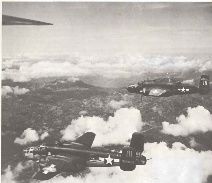
17. The red tips to the vertical tail surfaces identify Mitchells of the 321st BG: the nearest is 43-28082, a B-25J-5-NC version, and the second is B-25D-30-NC number 43-3522. The white roman III on the tail further identifies the 447th BS. (USAF)
