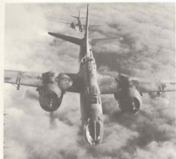
6. Bomb leader A-20J of the 410th BG; while 90 per cent of the 9th AF Havocs were solid-nose A-20Gs and A-20Hs with six forward-firing 0.50 machine guns, the transparent-nose A-20Js and A-20Ks proved valuable lead bombing aircraft over frequently overcast ETO targets. (USAF)
