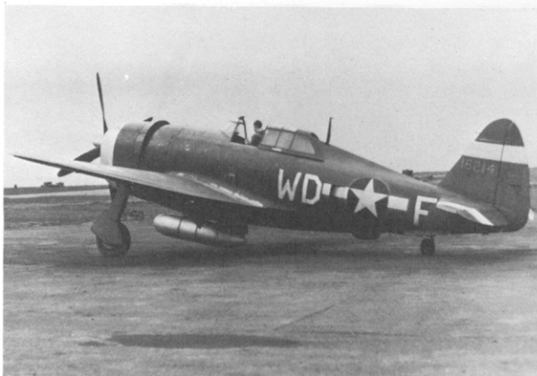
23. P-47C-2-RE (41-6214) of the 335th Fighter Squadron, 4th FG, Eighth Air Force carrying a 108 US gallon paper tank beneath the fuselage. Markings are standard for the period (the 4th FG flew Thunderbolts from March 1943 through February 1944) and include white identification bands on the front of the cowling (24in width), around the vertical tail surfaces (12in width) and the tailplanes (15in width), and red-bordered national insignia. (USAF)
