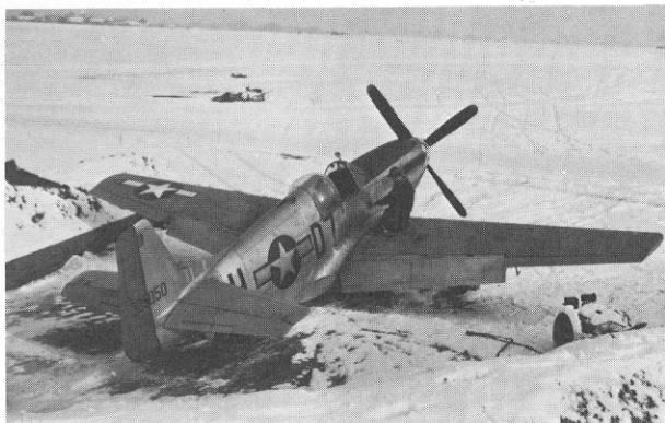
33. Photographed at Fowlmere on 2 March 1945, this P-51C-10-DT (43-25050) is fitted with a Malcolm hood and carries the red rudder and code (D7) of the 503rd Fighter Squadron, 339th FG, Eighth Air Force. The group markings consisted of a red-white-red ringed spinner and a two-row checkerboard in red and white around the forward 12 inches of cowling. (USAF)
