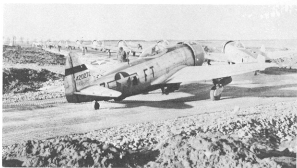
24. Bombed up P-47D-28-REs of the 353rd Fighter Squadron, 354th FG, Ninth Air Force, taxiing in preparation for a tactical sortie. Aircraft from this squadron had their cowling painted yellow. Note anti-glare panel extending fore and aft of the cockpit. (USAF)
