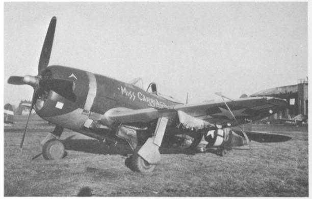
14. 'Miss Carriage', a P-47D-25-RE, photographed in England on 23 November 1944. Note large star-and-bar national insignia beneath port wing of this aircraft, a marking peculiar to Thunderbolts operating in the ETO which was applied to prevent the radial-engined P-47 from being confused with the German Fw190. (Robert Baseler)
