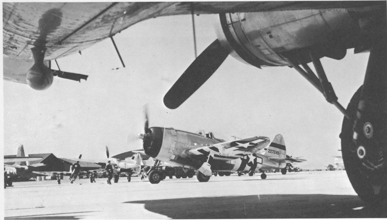
22. Typical scene at a USAAF base depot in England with a P-47D-27-RE (42-27249) taxiing between a B-17G (foreground) and some P-38Js, a P-47D and an A-20G (background). The Thunderbolts in this photograph carry the red cowling band which identified the 56th FG since March 1944. (USAF)
