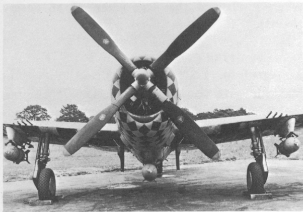
21. Front view of a Thunderbolt of the 353rd Fighter Group, Eighth Air Force, showing to advantage the devastating punch packed by this type of aircraft for short-range ground-attack sorties: two 1,000 lb bombs, one 500 lb bomb and eight 0.50 machine guns with 425 rpg. (USAF)
