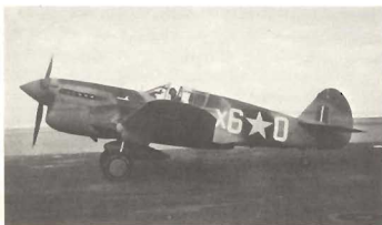
4. Second fighter unit to reach Africa was the 79th FG, late in 1942. The unit's P-40Fs had Olive Drab shadow shading over Sand and 41-14216 also has a toned-down fuselage star, along with the 'X' prefix to the aircraft number, which identified the group and the 86th FS respectively. (Via R. C. Ward)
