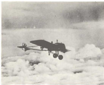
12. Pfalz E monoplane in flight; these were not nearly as popular as the Fokker machines of the same configuration, and the maximum number in use at the front was 56 at the end of April 1916.
