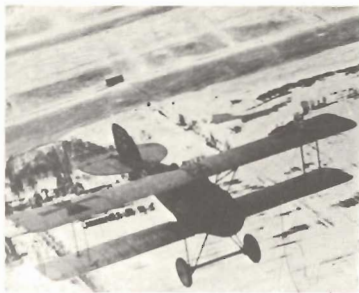
26. Leutnant Fleischer of Jagdstaffel 17 flying an Albatros D II over a wintry landscape. Note that this machine is not finished in the usual camouflage scheme, but apparently has natural linen-covered wings with national insignia without the usual 5 centimetre white surround.
