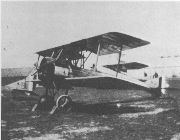
13. In June 1916 No. 60 Squadron used a number of Morane-Saulnier Type BB biplanes powered by 110hp Le Rhone engines. (Wg Cdr W. M. Fry)
