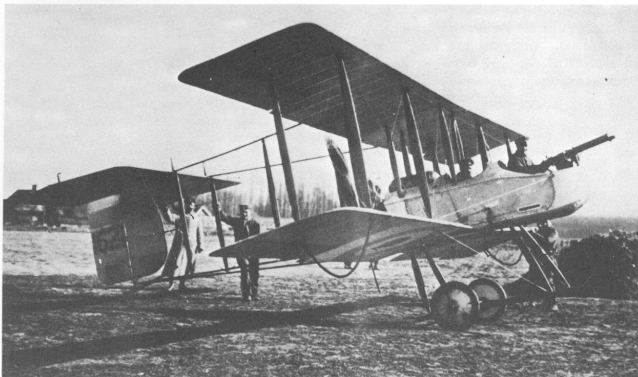
10. Vickers Gunbus No. 1621 in enemy hands. This machine was armed with a Vickers gun in place of the more usual Lewis and served with Nos. 2 and 16 Squadrons in February 1915 before being forced down intact in hostile territory. (Bruce/Leslie)
