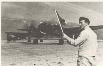
51. A pair of Ju88As being ordered to hold their take-off by the red flag in the hands of the 'starter'. When the runway is clear, a white flag with a green cross will wave the aircraft off.
