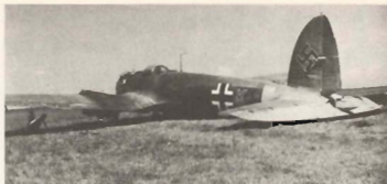
50. With the aid of jacks placed under the wings and fuselage, this He111H of 1 Staffel KG 53 is being raised from its belly landed position during the early stages of the Russian campaign. The aircraft, coded A1+KH, has a rearward-firing machine gun mounted in the tail cone.
