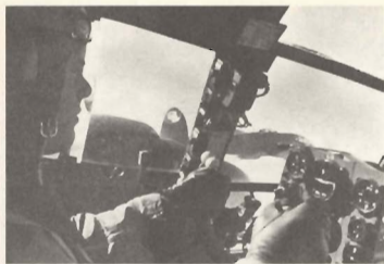
6. An excellent interior shot of an He111H showing the fine all-round visibility afforded by the fully glazed nose.
