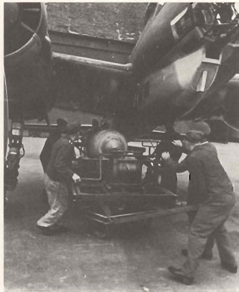
12. Limited internal space for offensive weapons meant that two of the three principal German bombers had to carry large-capacity bombs externally. Here, ground crews heave an SC1000 to the wing rack of a Ju88.
