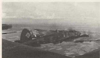
27. A photograph that well illustrates the effect of both weathering and overpainting of light areas with distemper on the fuselage of Heinkel He111H-16s of 8/KG 53.
