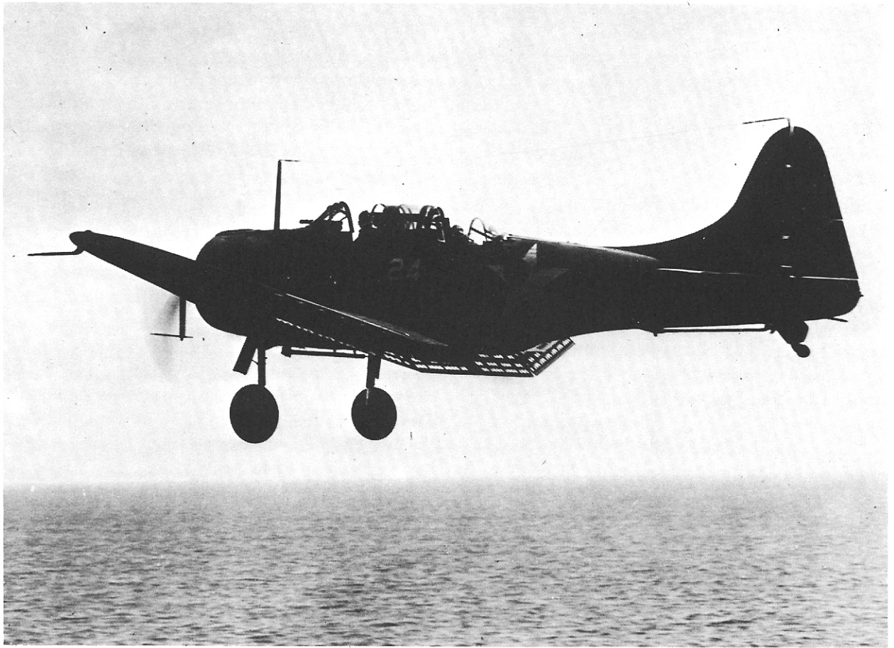
11. Douglas SBD-4 in landing configuration, with gear and perforated flaps down but hook still raised, approaching the USS Lexington (CV-16) on 23 April 1943. An interesting point here is that the red centre to the national insignia appears to have been applied in the wrong place.
