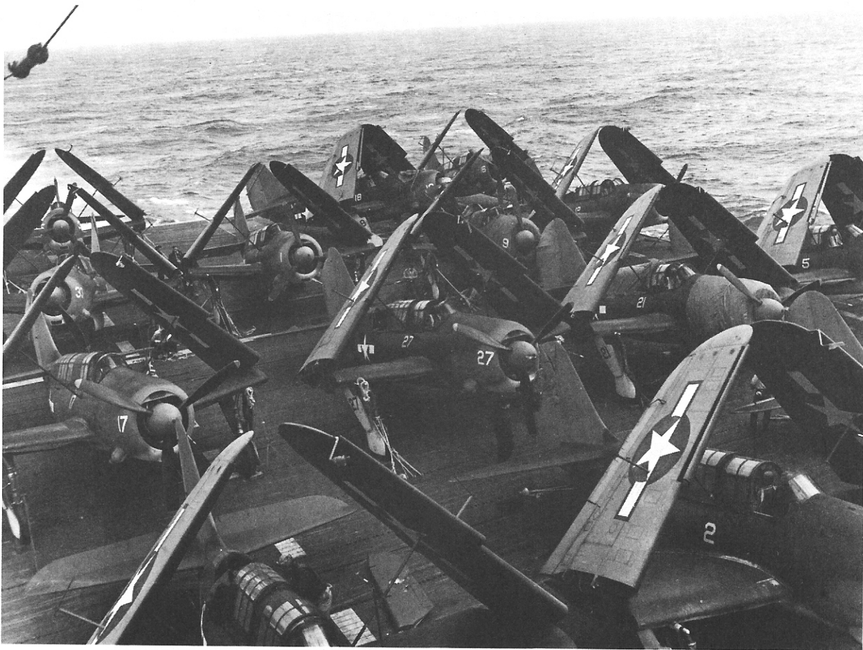
20. Curtiss SB2C-1C Helldivers of VB-2 on the aft deck of the USS Hornet on 15 February 1944. A heavy swell probably caused the visible rudder damage to aircraft 2, 27, 21 and 18 and a chewed-up elevator lies on the deck in the foreground.
