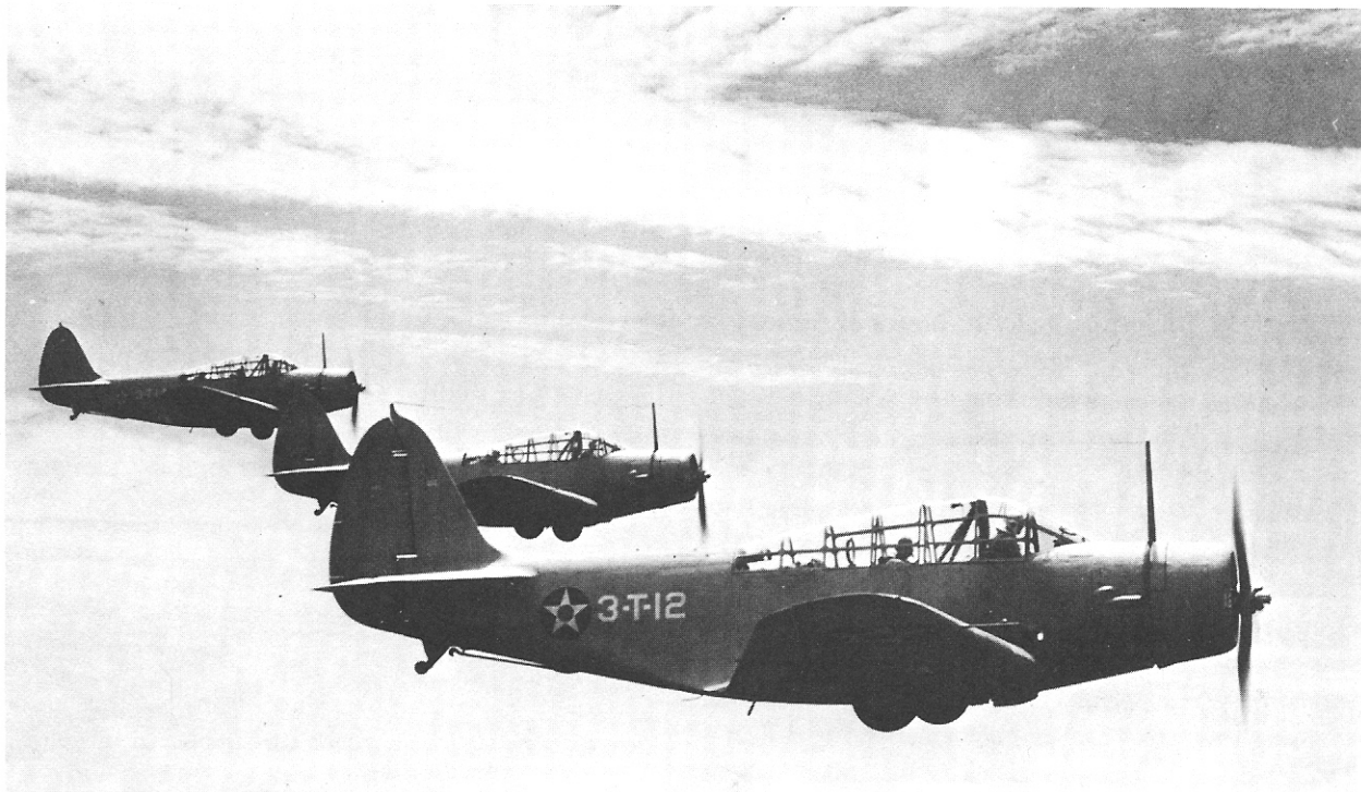
1. Douglas TBD-1 Devastators of VT-3 from the USS Saratoga in 1941. These aircraft are finished in the non-specular light grey overall specified for carrier-based aircraft during the 30 December 1940–12 October 1941 period.
