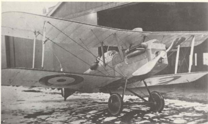
Lieutenant R. T. C. Hoidge in S.E.5 A4862 at London Colney in April 1917. The large windscreen, short exhaust pipes and non-adjustable radiator of the early S.E.5 can be clearly seen.
