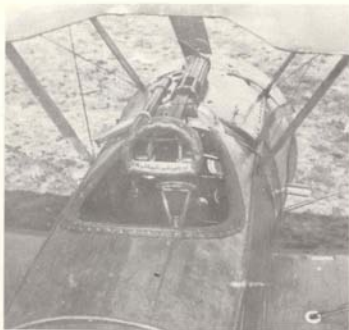
Cockpit of a Sopwith Pup showing the Aldis sight offset to port and the heavily padded end of the Vickers gun.
