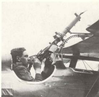
A Lewis gun pulled back on its Foster mounting on an S.E.5. To change the ammunition drum (not fitted here), the front of the gun was disengaged from its front wing clip by the pilot pulling a Bowden cable—which often resulted in a crack on the head as the slipstream forced the gun back too quickly. The remedy was an elastic bungee cord stretched between the barrel and the clip, enabling the gun to be pulled back under control. The cord can be seen running forward across the wing mounting. (L. A. Rogers)
