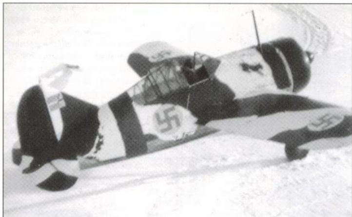
BW-362 'Orange 2' of 3/LLv 24 idles at Kontupohja prior to taking off. Within days of this photograph being taken, 5.5-kill ace Sgt Paavo Mellin was shot down in this aeroplane on 9 March 1942. He bailed out and was captured, remaining in captivity until Christmas 1944. BW-362's temporary winter whitewash consisted of glue and chalk mixed together, which was then brushed on in whatever pattern took the groundcrewman's fancy! (R Lampelto)
