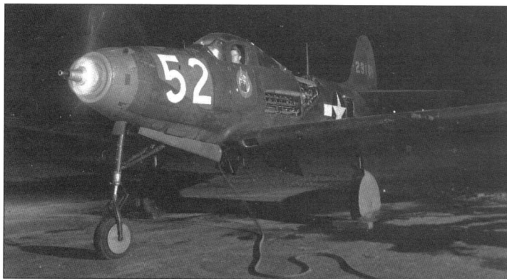
This night time shot shows a hardworking 355th FS groundcrewman running up the Allison V-1710 engine in his P-39N at Portland in September 1943. Night flying was a rare event for the 354th FG, so it is probably safe to assume that the airman is performing an engine test after carrying out routine servicing (USAAF)
