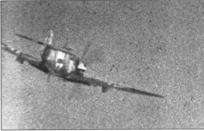
A scene that would be repeated hundreds of times over during the 354th FG's 18 months in combat in the ETO. This doomed rocket-armed Bf 109G has been caught by the gun camera fitted to an anonymous P-51B in the spring of 1944. The camera would automatically start filming as soon as the aircraft's 'fifties' were fired (USAAF)
