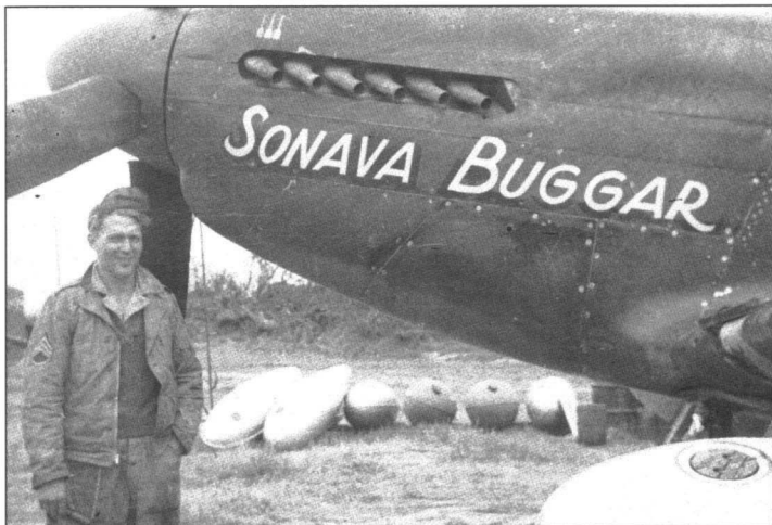
Crew Chief T/Sgt Paul Kempf poses nonchalantly alongside his P-51B in mid 1944. Sadly, the pilot of this amusingly named Mustang from the 356th FS remains unknown, as does the fighter's sub-type and serial. Note the three broom symbols above the exhaust stubs and the drop tanks piled up in the background (W Louie)
