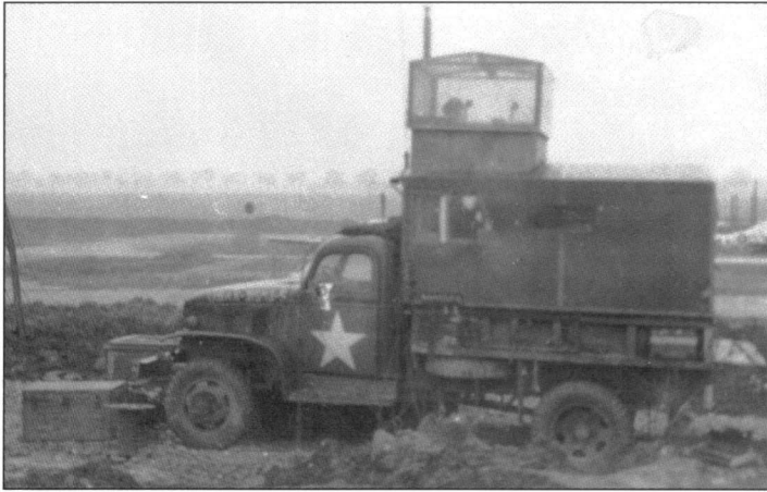
This Chevrolet G4100 1 1/2-ton 4x4 was used by the 354th FG as a mobile control tower in France. It is seen here surrounded by mud on a typically grey and misty day at Orconte (A-66) in late 1944 following the infamous flood ( W Louie )
