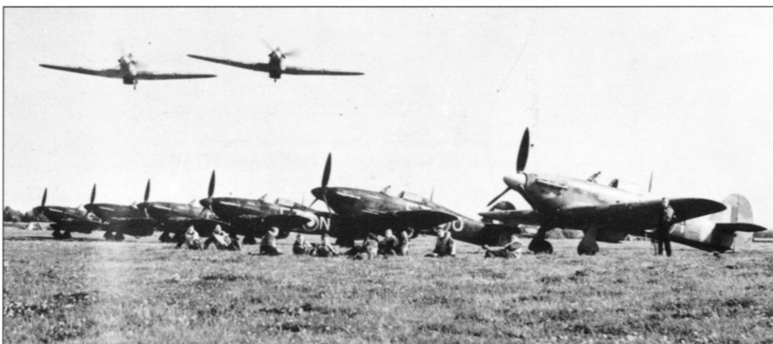
These line up shots of No 43 Sqn's Hurricane IIs at Tangmere in August 1942 are interesting in that they show the two camouflage schemes in use on the squadron at the same time – the temperate day fighter scheme (foreground) and the night black Intruder scheme in the distance. The first aircraft is Z3684 FT-L, flown by Plt Off R Barker during the Dieppe operation. Further down the line is BP703 FT-O in which Plt Off Snell was shot down over Dieppe (IWM)
