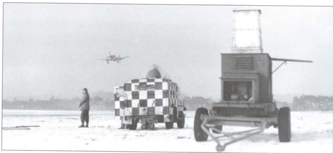
Mobile Landing Control is seen in action at East Wretham during the winter of 1944-45. The observation bubble atop the chequered vehicle appears to be a Plexiglas nose fairing souvenired from a nearby B-17 base
