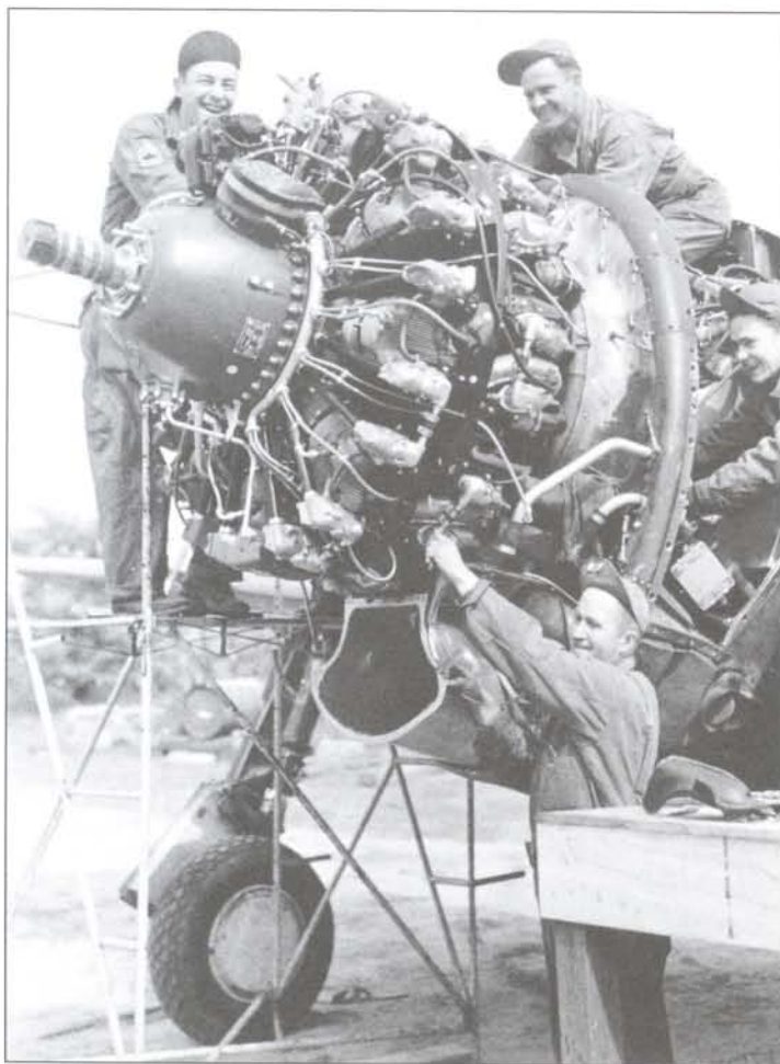
Initially plagued with gremlins, the big Pratt & Whitney R-2800 would duly prove both reliable and capable of running with entire cylinders shot away. Conducting a routine service on the line, these groundcrewmen are (from top left to lower right) T/Sgt Jack Linder, S/Sgt Earl Sneddon, Sgt Carrol Erickson and Sgt Chester Sawyer. As this photograph clearly shows, the P-47 was a big aircraft
