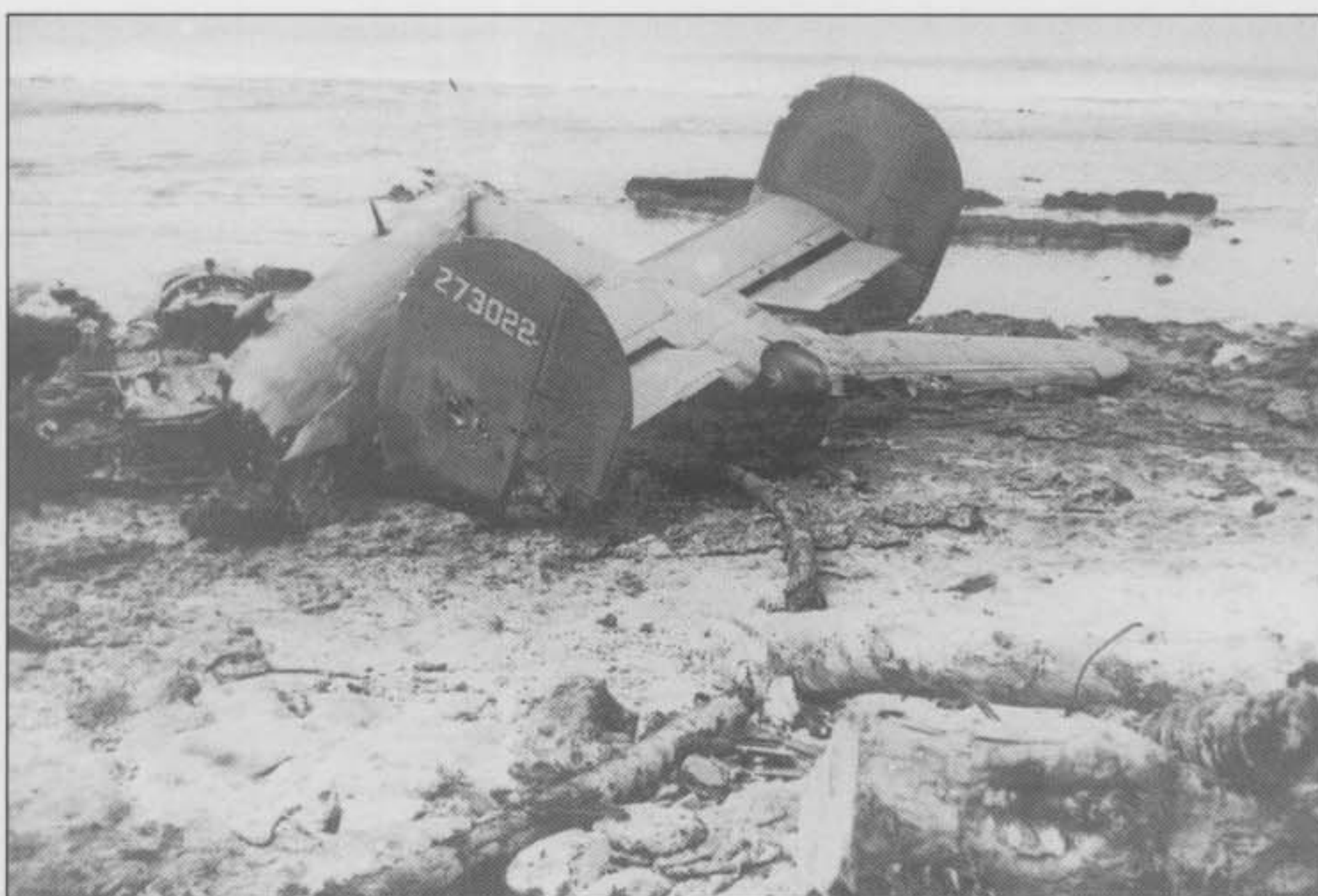
Hit by anti-aircraft fire during a strike on Jaluit, Lt Kurz's B-24J-5-CO (42-73022) of the 98th BS/11th BG – which never had a nickname – almost returned safely to Nukufateu on 23 November 1943. Hydraulic lines were shot out and there was a large hole in the wing under the no 1 engine. Unable to stop after touching down, the Liberator went off the south end of the runway and ended up some 150 ft (45 m) into the ocean, right-side up, in about four feet (one metre) of water. The aircraft was a total loss, but no one was seriously injured (via Bill Barstch)
