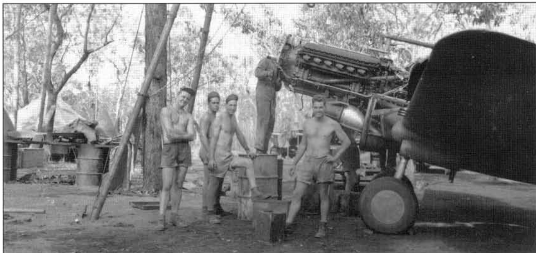
Long-suffering groundcrewmen pose for the camera while changing the engine of an 8th FS P-40E at Strauss Field in mid 1942. Note the total absence of maintenance stands and specialist servicing equipment (Steve Ferguson)
