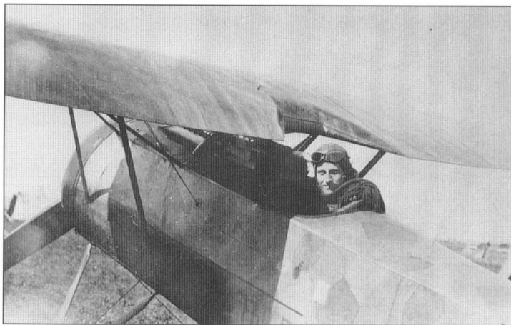
A Jasta 6 pilot thought to be Hans Reimers poses in the cockpit of Fokker E V 152/18 – Gefr Kurt Blümener was also photographed in this machine. This view emphasises the streaky quality of the dark camouflage applied to the plywood-covered upper wing (HAC/UTD)
