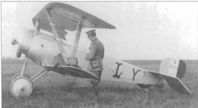
A visiting US Army officer examines Lufbery's Nieuport 21 N1615. A variant of the Nieuport 17 powered by an 80-hp Le Rhône engine, the Nieuport 21 was generally used as a fighter trainer only (National Archives)
