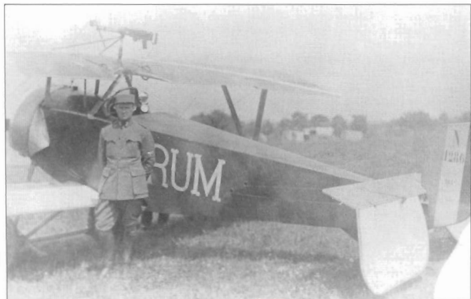
Sgt Lawrence Dana Rumsey Jr poses before his Nieuport 11 N1286 in July 1916. Note the light-coloured elevators and left lower wing – probably replacements for the damaged originals (H H Wynne)
