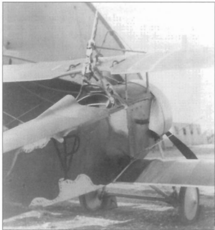
A close-up of Pavelka's Nieuport 16, seen from the other side, shows interesting details of the cockpit arrangement, the overwing machine gun mounting and the Lewis gun, with its ammunition drum removed (National Archives)
