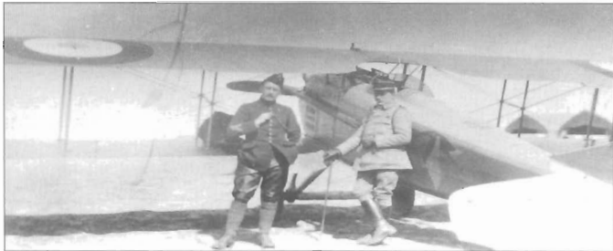
Dorme (left) at Bonne Maison beside his last SPAD VII, S392 'Père Dorme', which had the 180-hp Hispano-Suiza 8Ab engine. He first tested it at Le Bourget on 4 April and took possession on the 8th. 'My pressurised aircraft, which is tuned well, gives me absolute confidence,' Dorme said, scoring six victories in it before being killed on 25 May, the fifth victim of Ltn Heinrich Kroll of Jasta 9 (Louis Risacher album via Jon Guttman)
