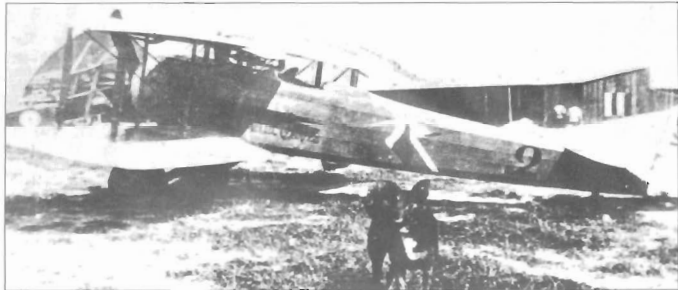
SPAD XII S382 was the new fighter armed with a 37 mm Puteaux cannon presented to Capitaine Guynemer at Saint Pol-sur-Mer in July 1917. Promising though it was, the SPAD XII proved to be a handful to fly, though Guynemer used it to score four victories whenever it was not undergoing repair (SHAA B76.1875)
