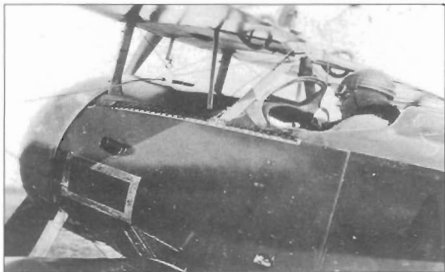
Sgt Georges Lutzius runs through some pre-flight checks in the cockpit of a Nieuport 17 of N103 in September 1916. This early Nieuport 17 had a Lewis machine gun on an overwing mounting, rather than the more common synchronised Vickers (SHAA B96.1276)
