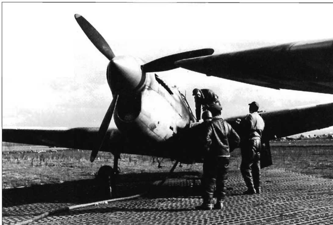
Groundcrewmen fuel a P-40 Warhawk nicknamed SWELL at Madna, in Italy, on 30 December 1943. The perforated steel plating runway seen here was commonplace at the group's various Italian airfields (National Museum of the USAF)
