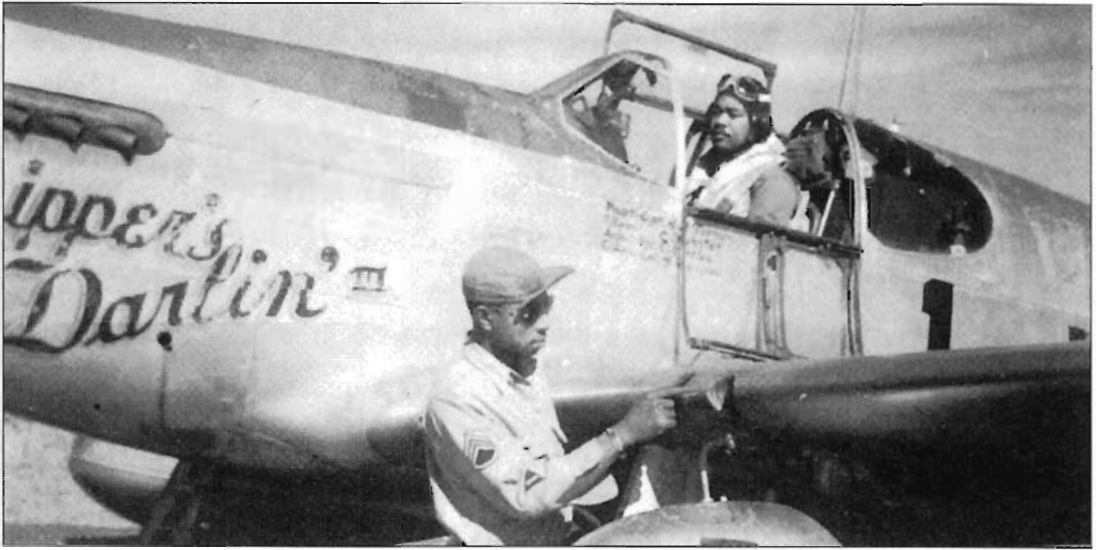
Another photograph of 'Jug' Turner's P-51C Skipper's Darlin' III , taken just prior to a mission in the autumn of 1944. Turner's crew chief appears to be applying a tape covering to the fighter's gun ports. This quick job was always done just prior to the fighter taxiing out, the tape helping to reduce the chances of moisture collecting in the barrels of the 0.50-cal weapons and then turning to solid ice at altitude, rendering the guns inoperable (Jon Lake Collection)
