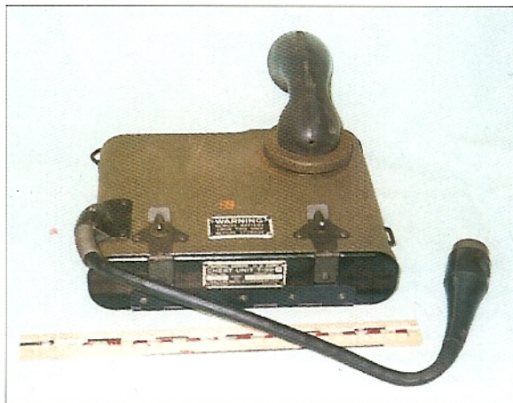
The SCR-511 "pogo-stick" radio was another small-unit voice radio used by Scouts and Raiders. It consisted of two components: the transceiver, with a support pole and a 4ft antenna (not pictured), and a chest pack (shown here) with the speaker to which the earphones were attached (not pictured). (William Howard, Technical Intelligence Museum)
