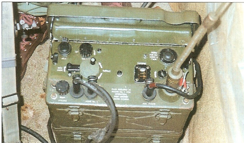
The SCR-300 "walkie-talkie" backpacked radio was used by both the Army and the Marines for voice communication between units, and to coordinate movements with delivery and recovery craft. (William Howard, Technical Intelligence Museum)
