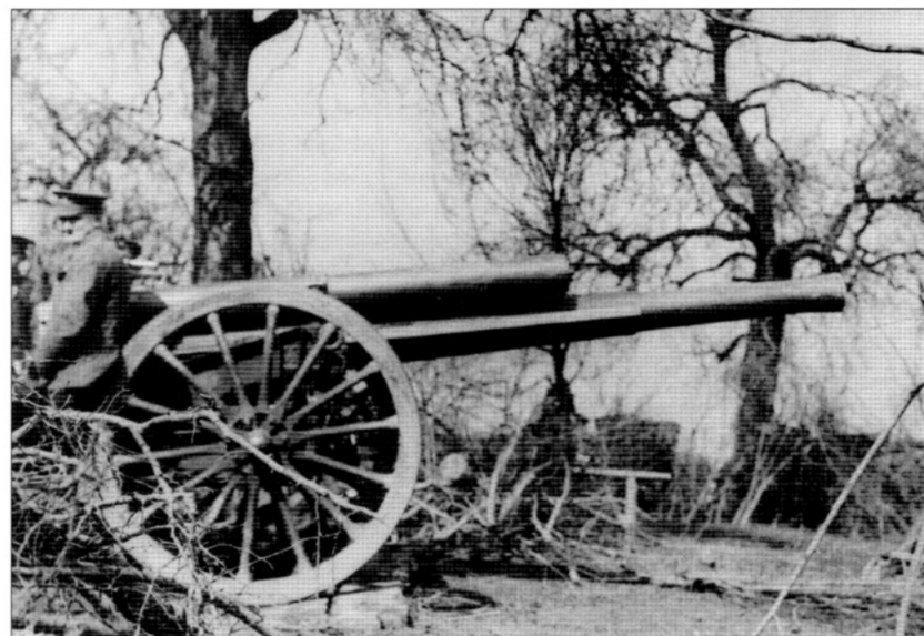
Though a vast improvement over the 4.7in. gun, the 60-pdr heavy gun was not without its problems. In the autumn of 1914 and the winter of 1915, broken recoil mechanisms kept many 60-pdrs out of the fight. The silver lining to this cloud was the effect that it had on ammunition supplies. Throughout the first year of the war, the 60-pdr was the only thoroughly modern artillery piece in the Expeditionary Force that was free from a chronic shortage of the right sort of shells. (Imperial War Museum, Q48940)
