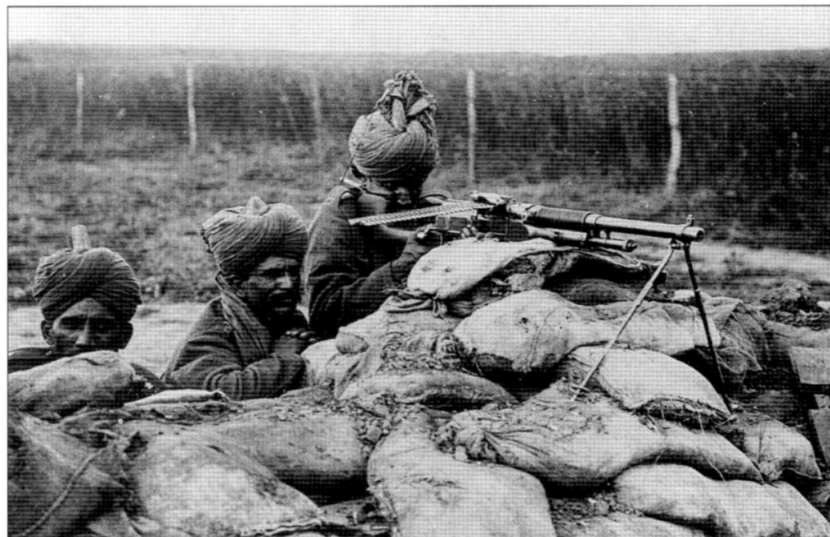
Most machine-gun sections serving with the Expeditionary Force were armed with either the old Maxim machine gun or the new Vickers machine gun. Some of the machine-gun sections of the Indian Corps, however, were armed with the Benet-Mercier light machine gun. A close cousin of the Hotchkiss machine guns that were soon to find a home in a number of British aircraft and tanks, this light machine gun fired the same .303in. ammunition as the other machine guns of the Expeditionary Force. (NARA)
