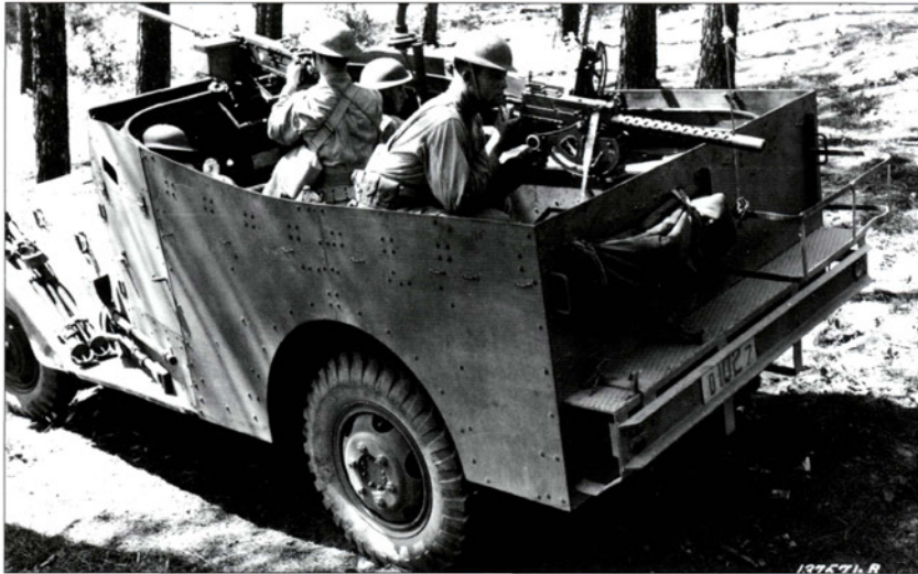
Members of Troop D, 102d Cavalry Regiment, in position and ready to fire from their M3A1 scout car during a practice reconnaissance exercise at Fort Jackson, SC. This car carries air-cooled M1919A4 light machine guns rather than the standard M1917A1 water-cooled guns. The radio operator operated one of the .30-cal machine guns; the other .30-cal and the .50-cal both had "full time" gunners. The M3A1 was the substitute armored fighting vehicle of the infantry division cavalry troop until the M8 armored car became available.
