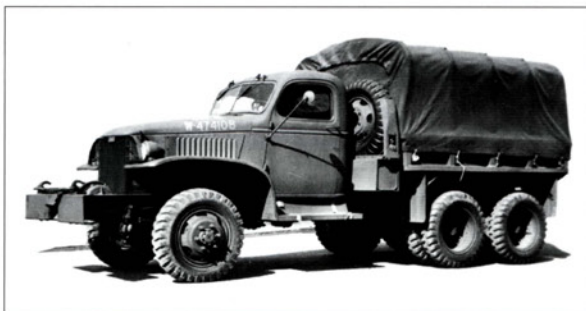
A CCKW-352 2 1/2-ton short wheel base (SWB) cargo truck with front winch; in an infantry division, SWB trucks mainly served as prime movers in the division artillery. Winch-equipped trucks often served as wreckers in 1942-43. Later production vehicles had soft-top cabs. (Recognition photo from about June 1942.)
