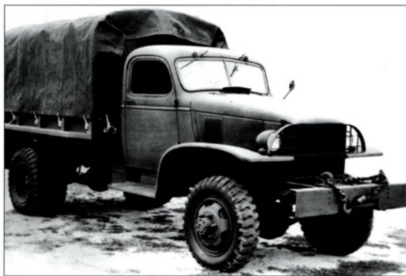
A G7117 1 1/2-ton cargo truck with hard top. (Recognition photo from about June 1942.)
