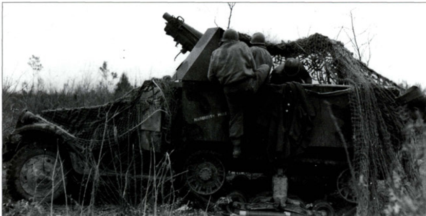
This uncaptioned photo shows one of the rare T30 self-propelled 75mm howitzers, with which infantry regimental cannon companies using the April 1942 tables were supposed to have been equipped. It is probably in combat in Italy, 1943.
