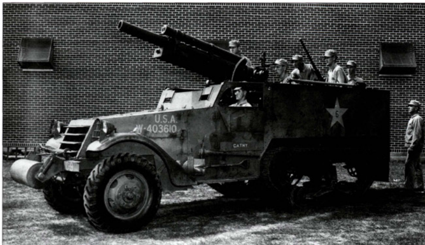
A T-19 self-propelled 105mm howitzer with .50-cal machine gun at a July 4th parade in Memphis Tennessee, 1942. In an infantry division this vehicle equipped the 105mm howitzer platoons of the infantry regimental cannon companies.
