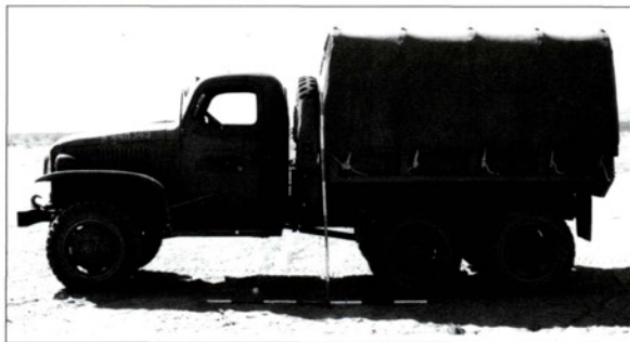
This identification photo shows a CCKW-352 2½-ton cargo truck (short wheel base) in side view. It was taken at the Desert Training Center, Indio, CA on June 8, 1942.
