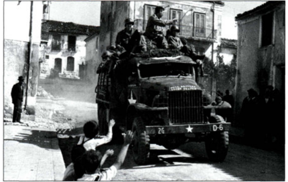
Townsfolk cheer as a CCKW-353 (long wheel base) with hard-top cab but no winch carries troops from the 180th Infantry, 45th Division, through Lioni, Italy, September 26, 1943.
