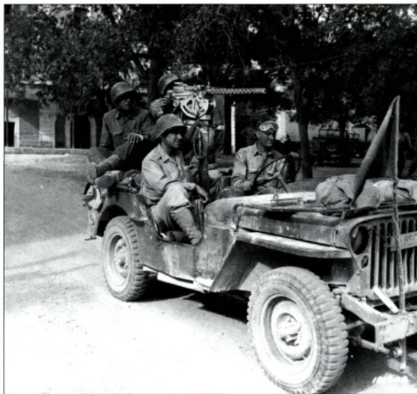
A jeep armed with an air-cooled M1919A4 LMG on an anti-aircraft type mount is pictured in southern Italy on September 27, 1943.
