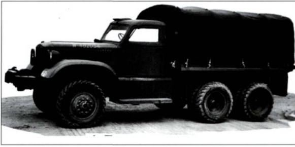
A Model 968A 4-ton cargo truck with hard-top cab and winch; in an infantry division 15 of these trucks served as prime movers for the division's twelve 155mm howitzers. Later production vehicles had soft-top cabs. (Recognition photo from about June 1942.)
