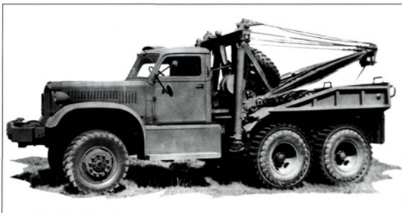
A Model 969A 4-ton wrecker with hard-top cab; this eventually became the standard light wrecker because the 2\frac{1}{2} -ton wreckers were not powerful enough. (Recognition photo from about June 1942.)
