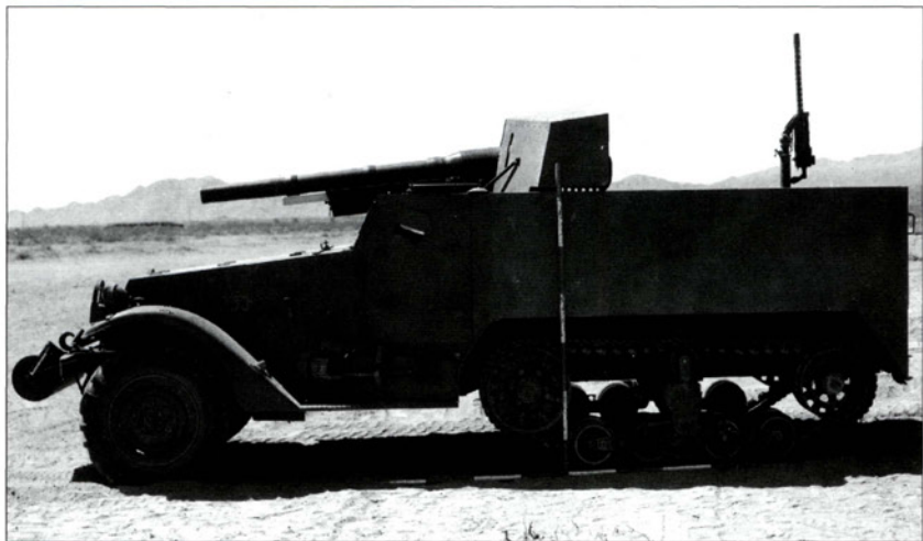
This identification photo shows a 75mm gun motor carriage M3 (or T-12) at the Desert Training Center, Indio CA (June 8, 1942). In the infantry division this was the most commonly used equipment of the 75mm platoons of the regimental cannon companies. This example also carries an M1919A4 LMG.
