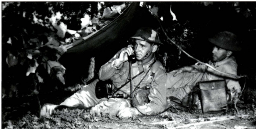
This uncaptioned photo shows an EE-8 field telephone in use, probably during a training exercise in the United States c. 1942.
