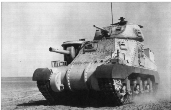
A Grant tank in the Western Desert, 17 February 1942. The US-made Grant tank proved a massive improvement over all British tanks in service when early models began re-equipping armoured units in Eighth Army in April/May 1942, in terms of armoured protection, reliability and firepower. Originally intended as an infantry support tank, the Grant had a curious design. The Grant had a turret-mounted 37mm gun similar to the Stuart Light tank, in addition to a 75mm gun in a hull sponson capable of firing both HE and AP rounds. This weapon at last gave tank crews a weapon that could outrange and penetrate the frontal armour on enemy tanks, as well as engage hostile anti-tank guns with a real prospect of suppressing or destroying them. A significant drawback, however, was the Grant could not engage from hull-down positions, and it had a very high profile making it also difficult to hide from view. (4700-32 E 8475)
