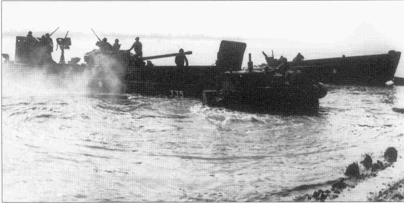
An American bulldozer pushes a naval landing craft containing an M18 MGC (Motor Gun Carriage) 'Hellcat', away from the near shore, prior to crossing into US Ninth Army's bridgehead. The silhouette of the Hellcat's long 76mm M1 gun can be clearly seen. The M18 was one of the finest tank destroyers of the war and saw action in both Italy and north-west Europe. (EN 59398, IWM)
