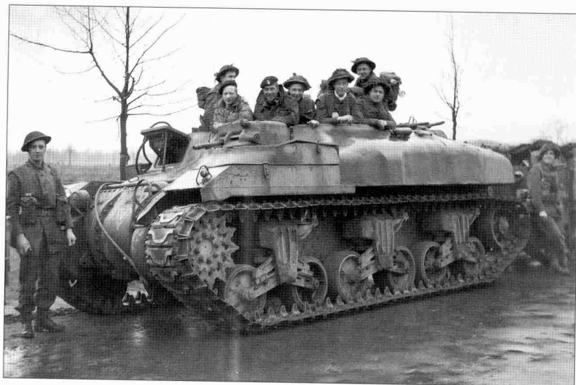
Troops of 53rd (Welsh) Division advance eastwards from the Rhine bridgehead in the relative security of a Kangaroo armoured personnel carrier provided by 79th Armoured Division. The carriers were modified Canadian built RAM tanks with turrets and associated equipment removed, allowing 11 fully laden troops to be carried. It had a crew of two men. (BU 2956, IWM)
