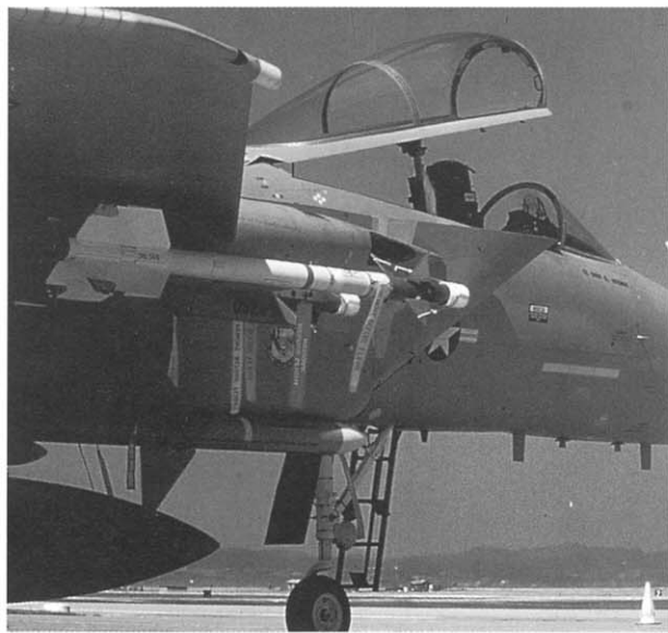
Above: Sparrow and Sidewinder missile locations are easily seen in this view of the forward fuselage of the Eagle. The large canopy area is also of note.
