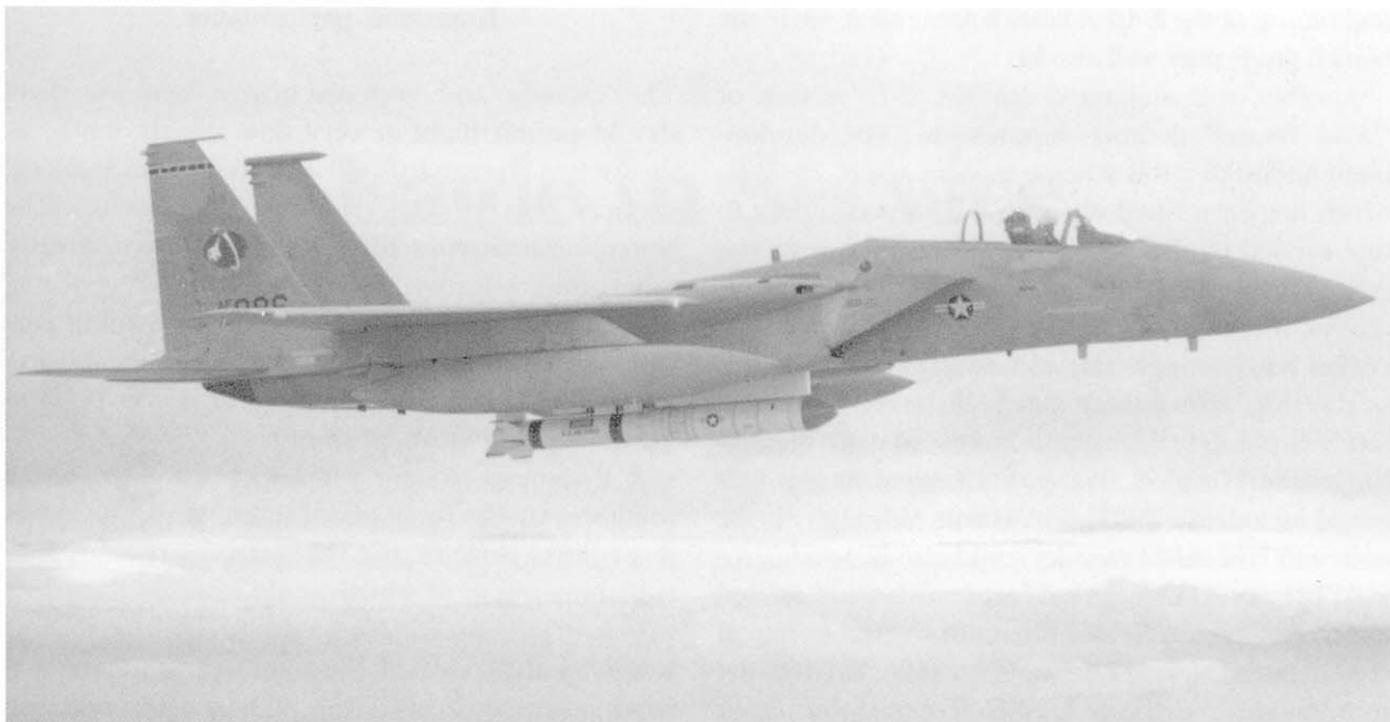
Above: One new role due to be undertaken by the Eagle is that of "satellite-busting". Here, Vought's ASAT weapon undergoes captive flight trials on an F-15A.
