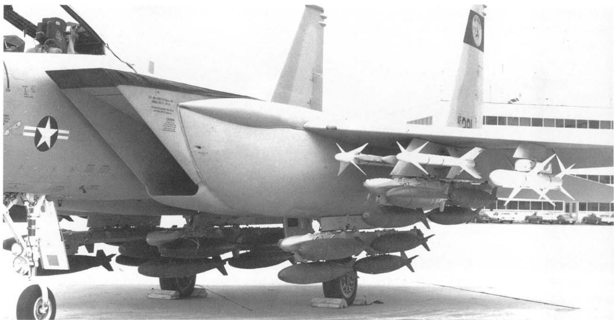
Above: This close-up of the stores stations of the dual-role fighter demonstrator shows it to be carrying conventional "iron" bombs plus AIM-9L and AGM-88A missiles.
