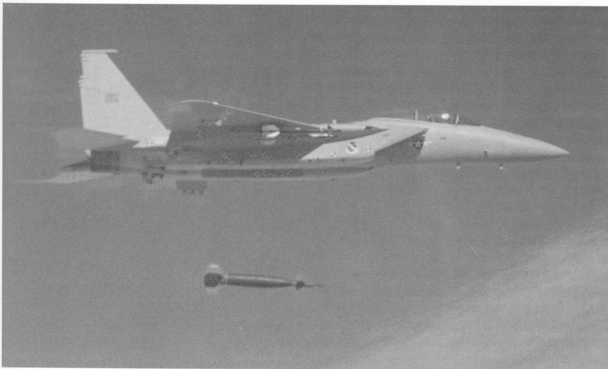
Above: One of eight full-scale development F-15A Eagles drops a laser-guided bomb during trials conducted by the Air Force Flight Test Center from Edwards AFB.
