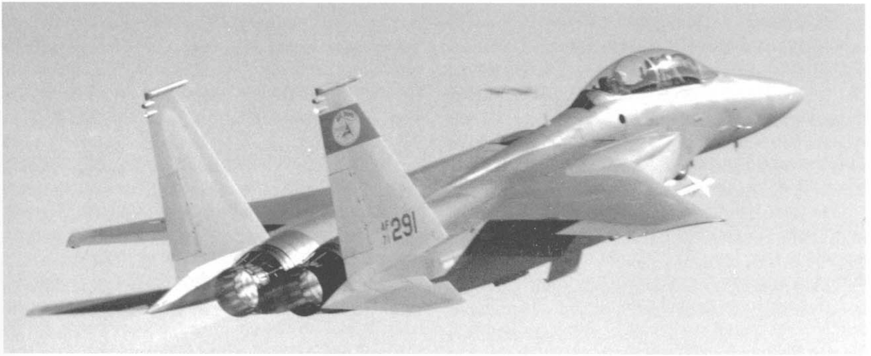
Above: Getting airborne in a hurry, MCAIR's two-seat demonstrator, 71-0291, clearly reveals the wide-set vertical tails and exhaust nozzles of the Eagle.
