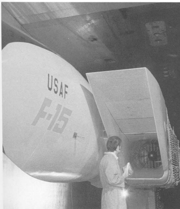
Below: Evaluation of the variable geometry air intake was long and thorough and included simulated flight at high speed in the supersonic wind tunnel facility at the Arnold Engineering Development Center. Here, a technician checks the intake prior to another test run.
