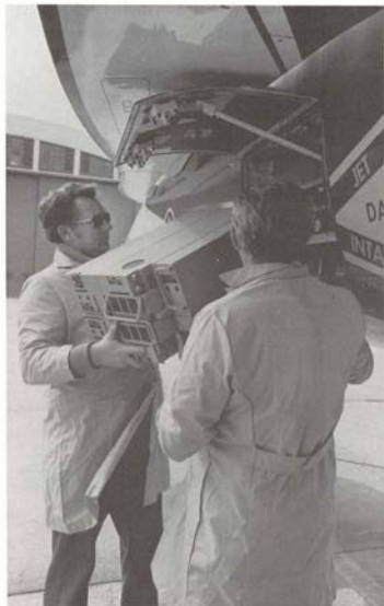
Below: The Sanders/Northrop ASPJ (Advanced Self-Protection Jammer) being installed on an FSD Hornet assigned to the Naval Air Test Center at Patuxent River.
