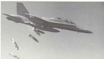
Below: Displaying the Aerospace Engineering Test Establishment's distinctive dayglo "X" marking on the fin, the first Canadian Armed Forces CF-18B (188901) delivers a batch of eight BL755 cluster bomb units during the course of weapons testing from Cold Lake, Alberta. Cameras mounted beneath the fuselage and wing tips recorded the drop for subsequent analysis by AETE.
