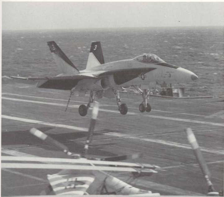
Above: Carrier suitability trials were predominantly the preserve of the third FSD Hornet, Bu.No.160777, seen here moments before "trapping" aboard the USS Dwight D. Eisenhower in February 1982.
