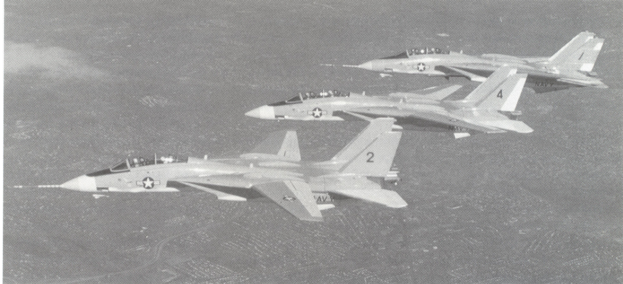
Above: With wings swept at differing angles, three of the dozen research, development, test and evaluation Tomcats fly in formation above a densely populated part of Long Island.
