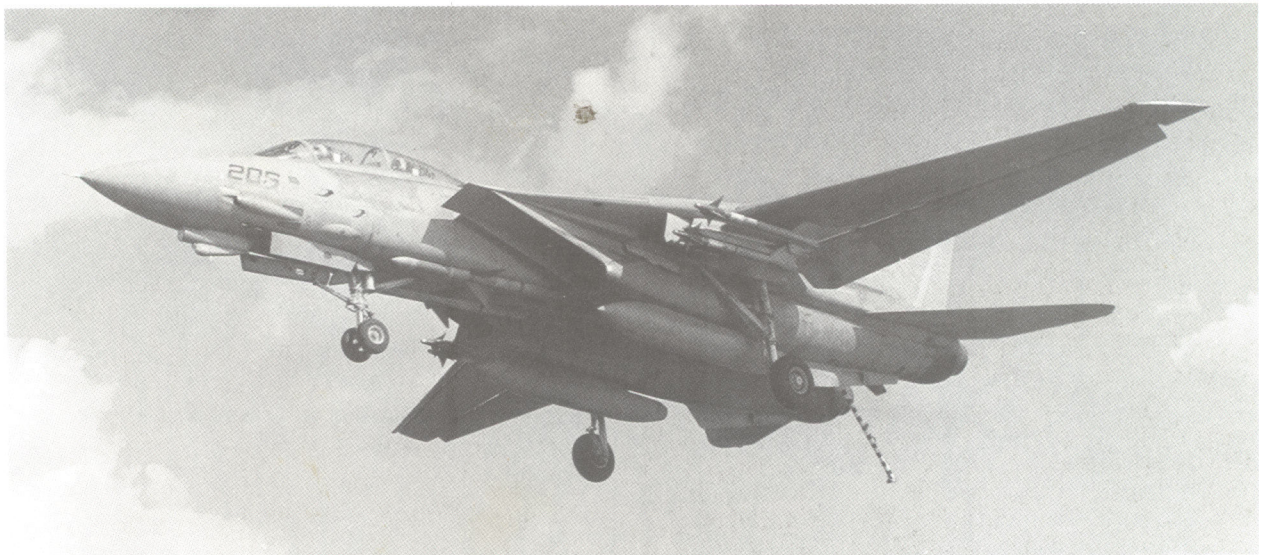
Below: Carrying a quartet of Sidewinders and two AIM-7 Sparrows, a VF-103 F-14A trails its arrester hook in anticipation of recovery aboard the USS Saratoga .
