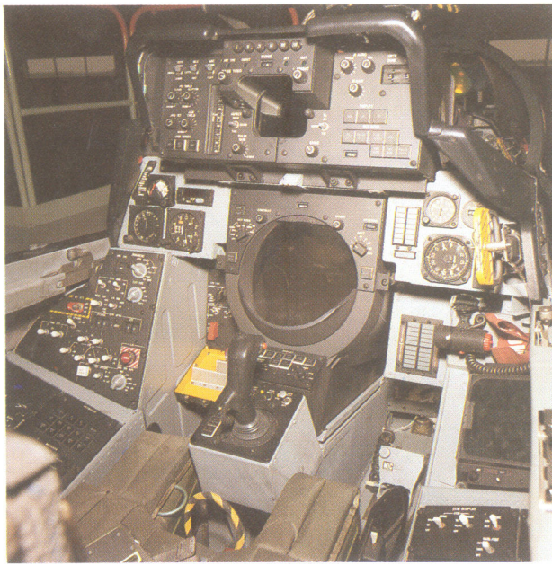
Below right: The Radar Intercept Officer's cockpit differs markedly from that of the pilot, with perhaps the most notable feature being the circular tactical information display and the adjacent hand control stick.
