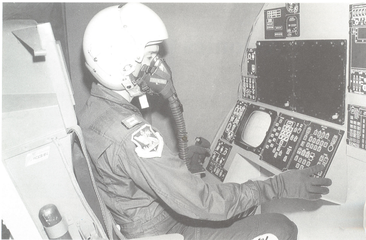
Above: Looking much less “busy” than the cockpit, the defensive systems operator’s station is nothing if not deceptive, hidden computers displaying data to the DSO by means of multi-function cathode ray tubes, with touch controls.
