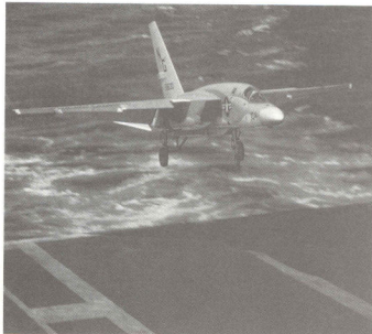
Below: The characteristic nose high Vigilante landing attitude is evident in this view of an RVAH-7 RA-5C returning to the USS Enterprise after a mission over North Vietnam in April 1966.
