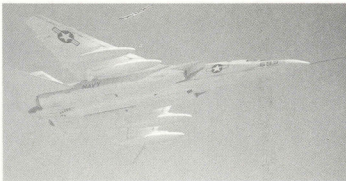
Above: Another view of the RA-5C aerodynamic test bed. The sensor canoe is clearly visible beneath the aircraft's belly as are the four underwing 400 US gallon jettisonable auxiliary fuel tanks.
