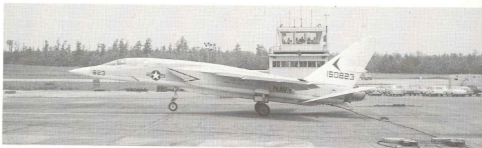
Above: RA-5C Vigilante 150823 of the NATC's Flight Test Division snags the wire during the course of arrestment trials at Patuxent River. This aircraft spent its entire service life with the NATC.
