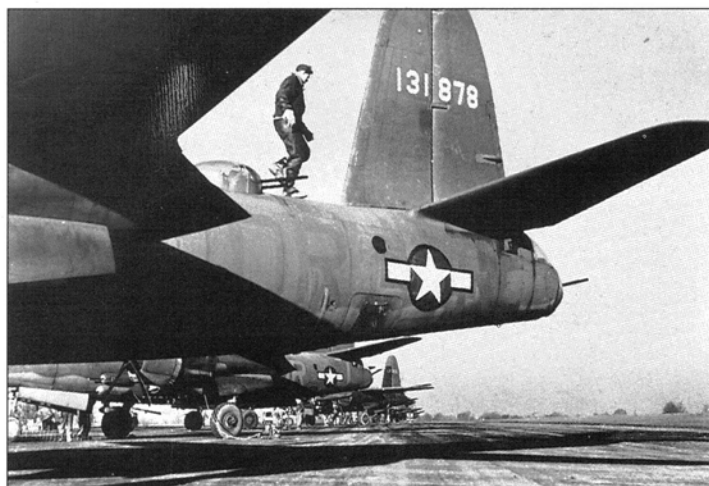
Flightline scene at 'Andrews Field', with Marauders of the 452nd BS being prepared by the hard-working groundcrews. Note how the grey paint used to pick out the code letters has become almost illegible against the streaked and weathered camouflage of the fuselage. This aircraft has also had the red 'star and bar' surround over-painted with fresh insignia blue, giving it an unusually dark outline (D Brett via MacKay)
