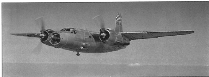
An off-photographed aircraft was B-26F-1 42-96246 of the 559th BS/387th BG, coded TQ-H. This bomber has had its nose cone armament deleted (Bruce Robertson)
