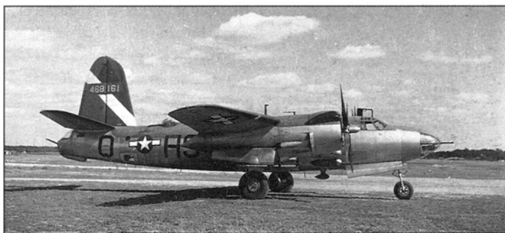
A well posed portrait of B-26G-25 44-68161/H9-Q of the 586th BS/394th BG at Villacoublay – one of the Paris airfields – in April 1945. The aircraft has the rear fuselage tray fitted to collect empty shell cases from the rear gun position, a modification that seemed to be rarer on Ninth AF Marauders than those of the Twelfth (H Holmes)
