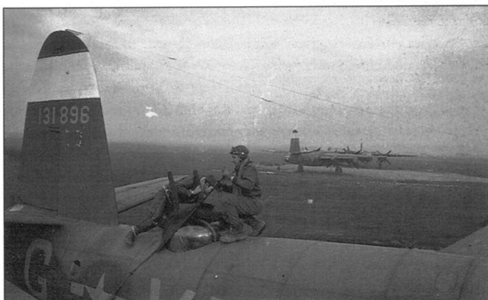
Misty English mornings rapidly lost their charm for young Americans when the daily round meant getting up just to go out and be shot at! At Marauder bases such as Earl's Colne, custom-made covers prevented that all-pervading damp from getting into turret and gun mechanisms. Here, aircraft of the 453rd BS await the fuel bowser as two members of the flight crew, rather than groundmen, prepare their bomber's primary defensive position for combat (John Hamlin via R MacKay)
