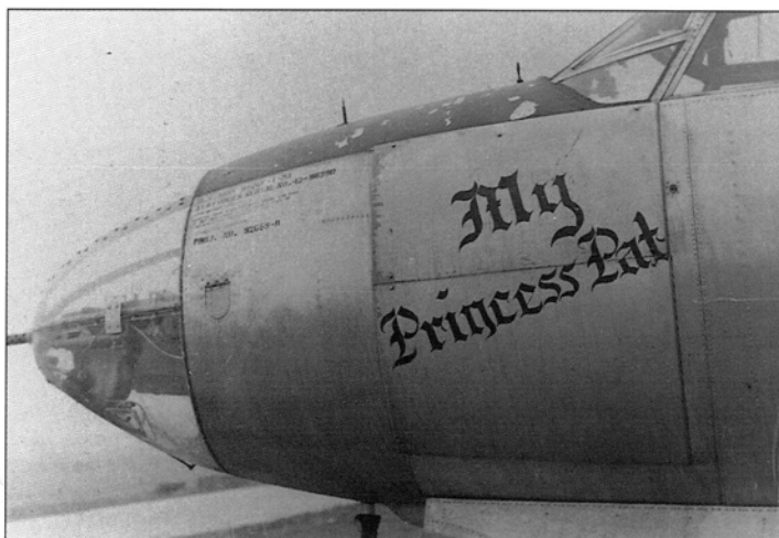
A close up of the nose of B-26F-1 42-96290, featured on the previous page. This view clearly shows the additional applique armour plating fitted in order to better protect the pilot from flying shrapnel, as well as the twin aerial location points forward of the windshield. Salient details of the Plexiglas nose section, with its centreline .50 cal machine-gun and associated bag for collecting empty shell cases, are also clearly visible (Crow)
