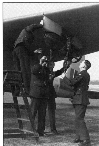
Armourers fit a 250-lb bomb to the wing of FB VI LR355/'H' of No 613 Sqn. This aircraft was still serving with the unit when it was written off in a crash-landing following an engine failure on 1 August 1944
