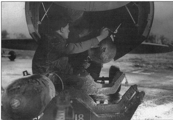
An armorer hoists a 500-lb bomb into position aboard an FB VI during the winter of 1944-45. This Mosquito variant could carry two 500-lb bombs in the rear half of the bomb bay only, as the forward half was taken up with cannon breeches (via GMS)
