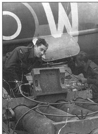
No 613 Sqn's AC1 Phillip Beck and LAC E Kerlake – the 'boys with the gen' – refill FB VI 'W's' oxygen tanks in preparation for a raid on Berlin (Flight via Phillip Beck)
