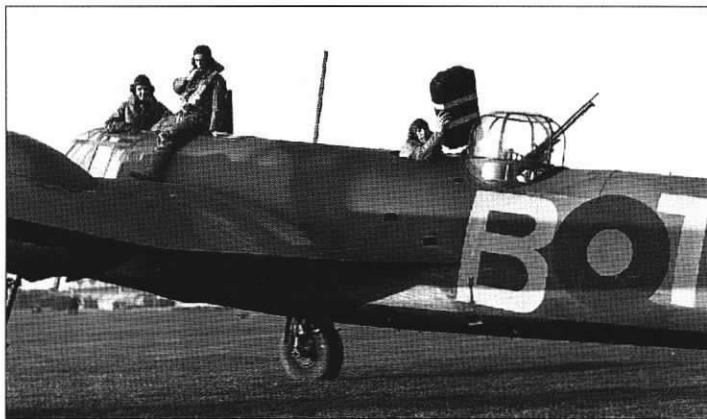
Generations of aircrew have undertaken the faintly ridiculous charade of practising their ditching drill on dry land. Here the crew of a No 90 Sqn Blenheim I try to take it all seriously, as the gunner throws the dinghy pack onto Bicester's grass. The aircraft bears obvious traces of having had its A1 roundel toned down and converted to a B-type roundel. The steps for the aircrew are clearly visible above and below the wing trailing edge (via Aeroplane )
