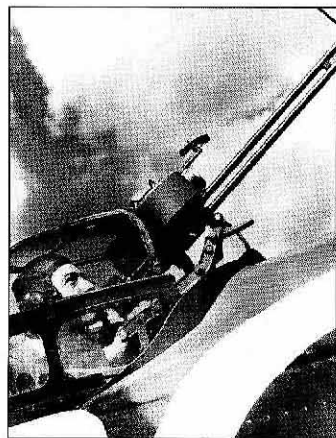
A Blenheim gunner poses for the official camera, crouched behind his VGO machine gun. Even with a power-operated turret, a single 0.303-in gun was little better than a peashooter against a 20 mm cannon armed Bf 109 (Aerospace Publishing/Wings of Fame)
