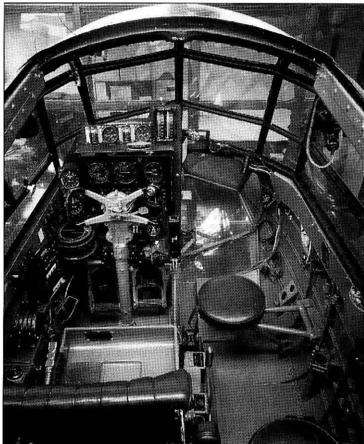
The cockpit of a Blenheim I, with the observer's seat folded down beside the pilot's. No bombsight is fitted, and the aircraft has no ring-and-bead gunsight, indicating that the photo was taken at the factory, before completion. The aircraft has a full blind-flying panel, and has an old-fashioned 'flat' compass. The extent of the aircraft's nose glazing is readily apparent ( Aerospace Publishing/Wings of Fame )
