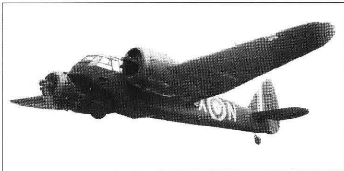
The wartime censor obliterated the underwing radar antenna on this photo of K7159 (see on the previous page), but left the overwing and nose-mounted antennae. The individual aircraft letter 'N' was outlined in yellow, denoting the aircraft's assignment to an OTU (Aerospace Publishing/Wings of Fame)
