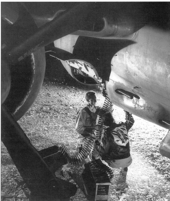
The gunners in the 6th NFS held a dual role, for they not only loaded the guns but fired them as well. Facing the camera is Sgt Jerry K Lucas, whilst squadron artist Sgt Leroy Miozzi, wearing the painted jacket, has his back to the camera. Both veterans of numerous missions over the Pacific, they are seen here loading 20 mm rounds into the belly magazine of a squadron Black Widow (USAF)
