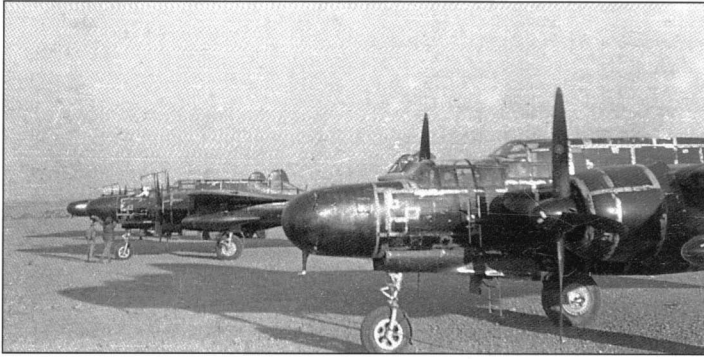
This line up shot was taken on 3 March 1945 following the delivery of the first P-61s issued to the 417th NFS to the unit's base at Lavallon, in France. The aircrafts' pristine all-black finish had been marred during post-shipping re-assembly by the removal of the protective tape from the airframe joints, leaving bare metal to show through where the paint had come away (Richard McCray)
