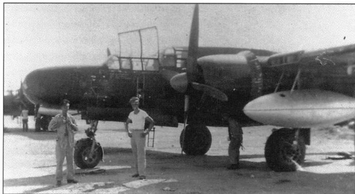
2Lt James W Schuler and his R/O Fit Off Arthur D Miller take a look at the new 310 gal tanks that have been recently attached to the pylons of their P-61. The 550th NFS began using the stores to fly long-range night intruder missions, the tanks weighing in at around 2000 lbs apiece when full ( Newell Witte )
