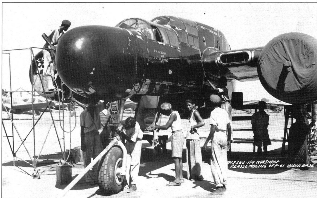
A brand new P-61 is unloaded, uncrated and prepared for service (with either the 426th or 427th) at an assembly centre in India. Note that the ADF antenna has not yet been installed on top of the crew nacelle (Garry Pape)
