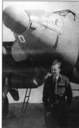
FB VI PZ459 was assigned to 'A' Flight of No 515 Sqn at Little Snoring, where it was coded 3P-D 'D-Dog' and flown almost exclusively by Plt Off Leslie George 'Dutch' Holland (pictured) and Flt Sgt Robert 'Bob' Young. Note the Al Mk XV ASH (Air-Surface H) nose radome – ASH was designed as a wing-mounted radar, but it was found to be unsuitable for fitment to the Mosquito's slender wing, so it was installed in a 'thimble' radome in the nose instead. Following service with No 515 Sqn, PZ459 was briefly used by No 141 Sqn before being placed in storage. It was eventually sold as scrap in July 1947 (Leslie Holland via Tom Cushing)
