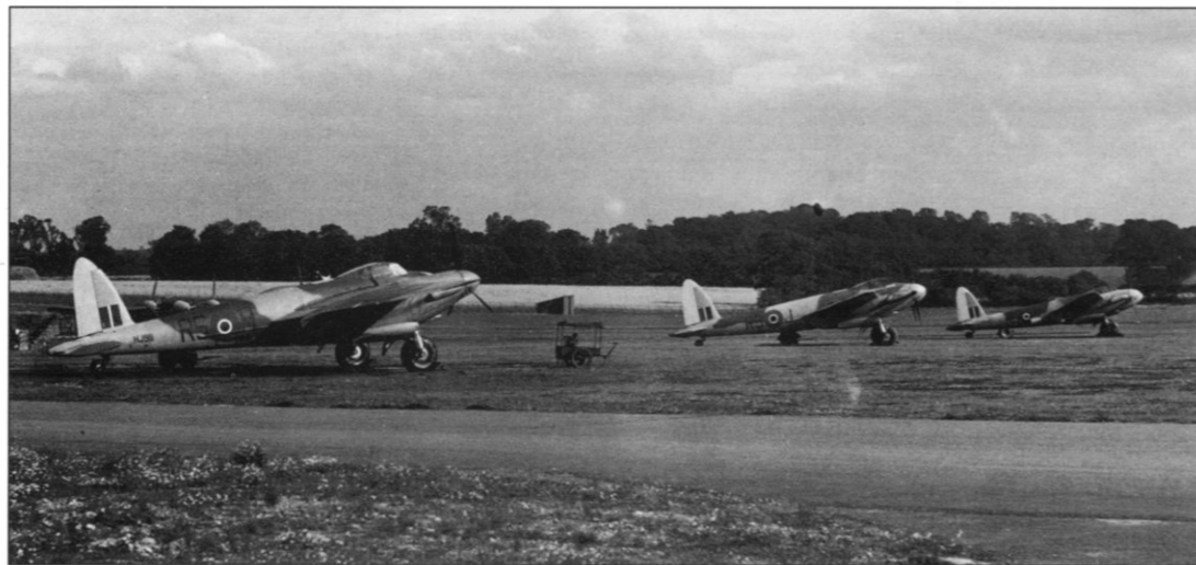
The NF IIs used by No 100 Group units in December 1943 had previously seen much use with Fighter Command, and serious reliability problems were experienced both with their Merlin 21s and AI radar. This photograph shows NF IIs of No 157 Sqn at Swannington in May 1944, with Leavesden-built HJ911 parked nearest to the camera. As the first in a batch of 34 NF IIs delivered to the RAF between September and November 1942, this aircraft had served with No 157 Sqn for almost two years by the time this shot was taken, and it went on to serve with Nos 141 and 307 Sqns and No 1692 Flt before being struck off charge on 19 February 1945. Its sole nocturnal success came on 27/28 June 1944 when No 141 Sqn's Sqn Ldr G J Rice and Flg Off J G Rogerson destroyed a Ju 88 over Cambrai
