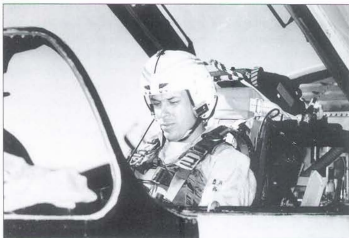
Back in the cockpit following his return to the States, Lt Klusmann prepares for his first flight. Note the rocket-jet fittings on his shoulder straps, and the V-ring on the right strap, which served as a hook-up point for a rescue helicopter's hoist
