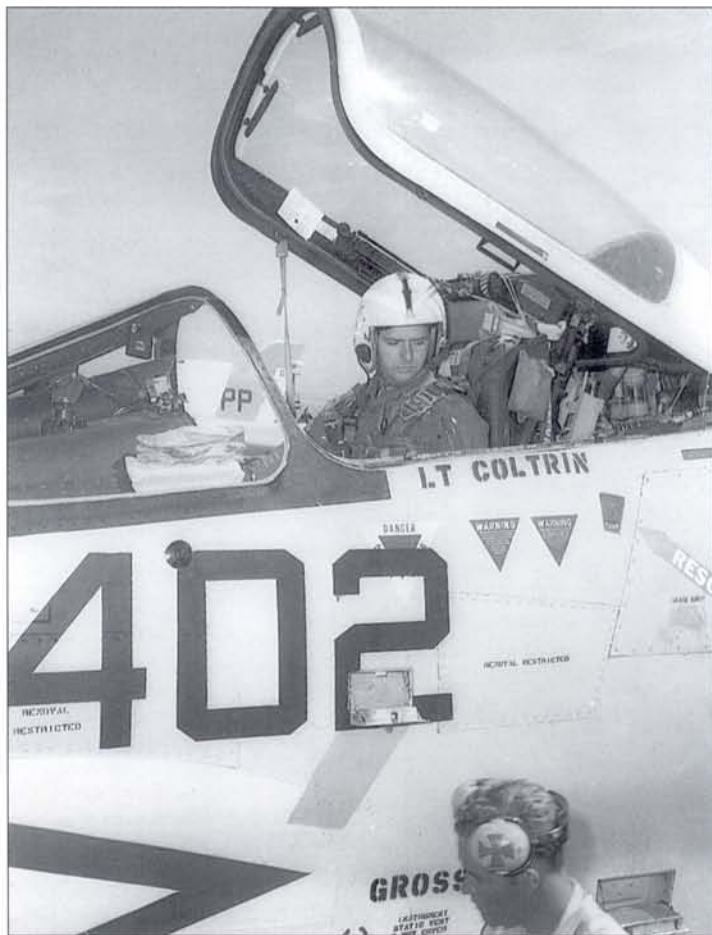
Lt Andre Coltrin in an RF-8G during a carrier qualification period at NAS Miramar. His large white flight helmet features a dual-action knob in the centre that lowered one of two visors – clear or smoked – depending on the light. Note the cloth strap attaching the canopy to the fuselage, this simple device helping protect the canopy's hinge pins from breaking in wind gusts. The pilot also used the strap to pull the canopy down
