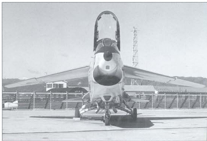
A head-on view of a Marine RF-8A showing the distinctly 'boxy' look of the redesigned fuselage, which deleted the fighter's cannon for the suite of cameras. The pilot's viewfinder window is directly below the black nose cone. The fairing directly above the nosegear houses the forward-firing KA-45 camera – one of the aircraft's primary sensors
