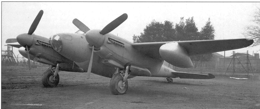
RG176, pictured in January 1945 with 200-gal wing drop tanks during trials at the A&AEE, was the first PR 34 and it flew on 4 December 1944. In May 1950 the aircraft was converted to a PR 34A by Marshalls, before being issued to No 540 Sqn at Benson, who used RG176 from July 1951 to June 1952, when, after an accident, it was reduced to spares by No 58 MU (DH via Philip Jarrett)
