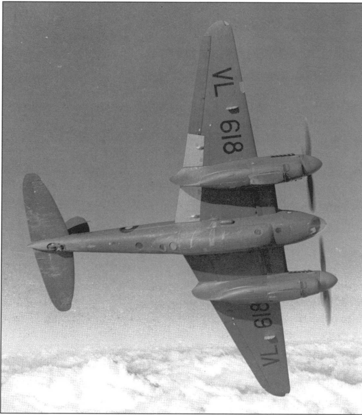
PR 34 VL618 in overall PRU Blue in flight, showing the five underbelly circular windows for vertical and oblique cameras. All PR 34s carried four split F 52 vertical cameras – two forward, two aft – of the belly tank, and one F 24 oblique camera (or, alternatively, a vertical K 17 camera for air survey) aft also (BAe via Jerry Scutts)
