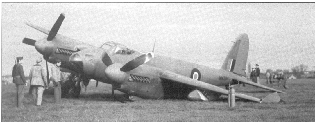
MM384 lost its port undercarriage during landing at Watton on 4 May 1944, being repaired on site, before being sent to Burtonwood on 8 July 1944 (via George Sesler)
