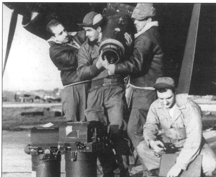
654th Sqn Photo Lab personnel show off their aerial cameras, which they operated from onboard Mosquitoes at Watton. Camera equipment used consisted of the Fairchild K series in the 6-, 12- and 24-in models. Also used was the British F camera with its 36-in lens. For BDA, the Fairchild K20 and K21 hand-held cameras were carried. The radar or Mickey camera which provided a photo log of radar imaging, used by the 654th BS, was a development of the Camera Repair Dept at Watton. via Ken Godfrey
