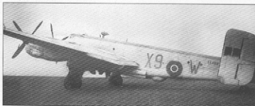
This Halifax Met V wears the 'X9' codes of No 517 Sqn, but is seen here in the Halifax graveyard at Rawcliffe immediately after the war. Unusually for a Meteorological aircraft, it has a Preston-Green turret below the fuselage (via Phil Jarrett)
