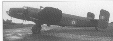
The final wartime Airborne Halifax was the A VII, shown here. The aircraft was basically an 'Airborne' conversion of the B VII bomber (Author's Collection)
