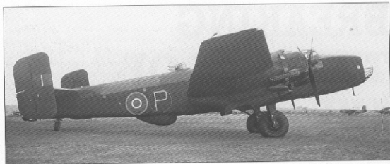
Although it wears the distinctive yellow 'prototype' marking, HX238 was an early-production B III retained for trials at Boscombe Down, and not the prototype. It is seen here with Hercules 100 engines, acting as a B VI prototype (Author's Collection)
