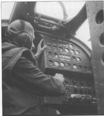
Sitting on a fold-away seat beside the pilot on take-off and landing, the flight engineer had his own panel behind the pilot's seat, allowing him to control the engines and fine-tune fuel flow and power (via Aeroplane )
