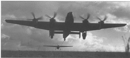
The A V was essentially a B V Series IA with a glider towing hook behind the tailwheel and a paratroop hatch in the lower fuselage (via Phil Jarrett)
