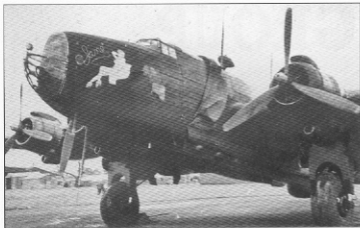
Jane (actually MZ913, coded Z5-N) was the aircraft of RAAF pilot Flt Lt Ron Hines, subject of one of the figure artworks in this book. The aircraft carries ABC aerial masts below the nose and above the fuselage, and small antenna fairings are visible along the bomb doors (Jerry Scutt via Martin Bowman)
