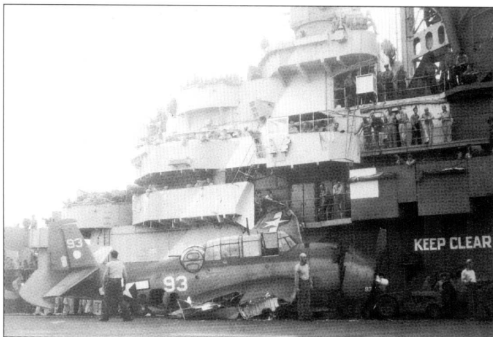
Ensign F T Long of Torpedo Squadron Two wrote off TBM-1C BuNo 45593 in a crash-landing aboard Hornet on 19 June. Number 93 had already sustained previous damage, attested by the still unpainted fabric patch on the rudder (Author's collection)
