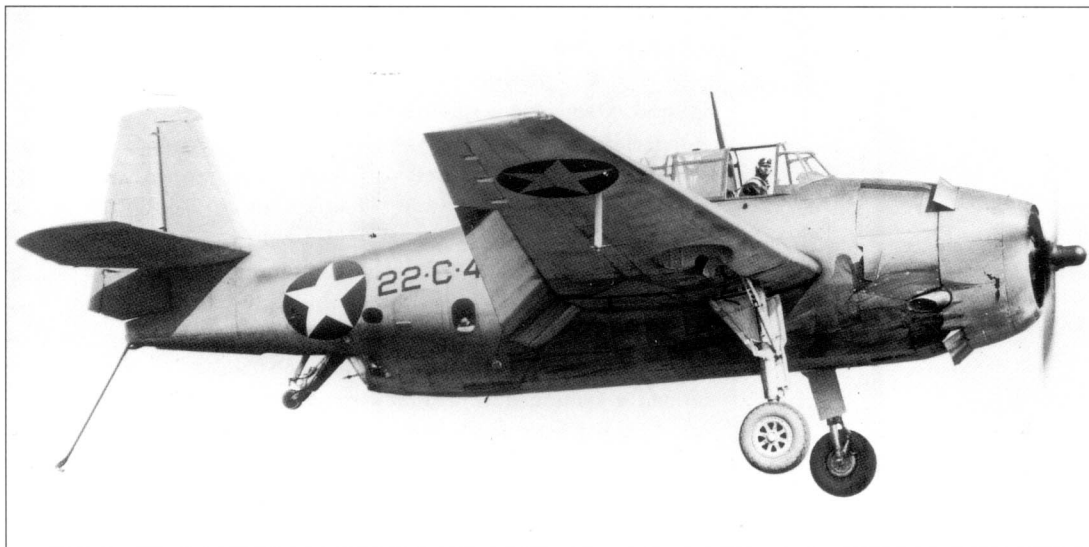
Naval colours in transition. Taken in May 1943, this photo depicts a VC-22 aircraft assigned to the light carrier USS Independence (CVL-22). An early version of the tri-colour scheme (white undersurfaces, medium blue sides and dark-blue upper) is offset with 'Stateside' unit markings and the cockade style star. Horizontal bars were added later that year ( Author's collection )
