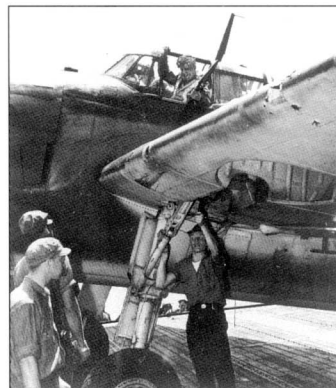
Lt Robert R 'Railroad' Jones deplanes after recovering safely back aboard Enterprise at the end of a rough mission over Truk on 16 February 1944. As Jones exits the cockpit with his cardboard, VT-10 crewmen survey the flak damage to his TBF-1C, which shows both entrance and exit holes in the leading edge of the port wing (Author's collection)
