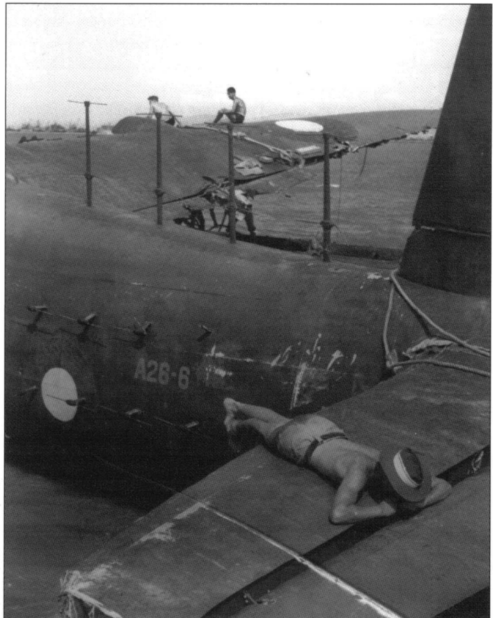
Photographs of the Sunderlands flown by No 40 Sqn RAAF are extremely rare, and have seldom been seen in print. The unit's aircraft wore an overall foliage green camouflage, with SEAC roundels and fin flash as seen here. This aircraft appears to have suffered serious damage both to its starboard wing trailing edge and port tailplane tip (via Phil Jarrett)
