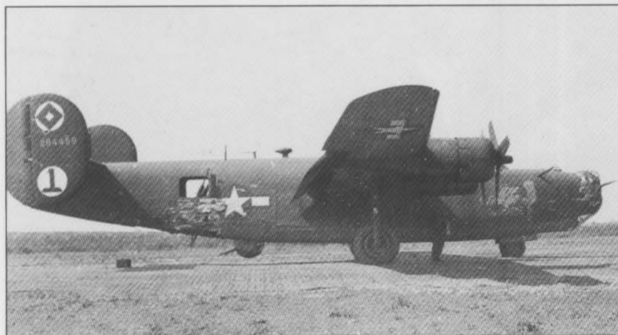
Below and right below Liberators of the Fifteenth Air Force had the most arcane, and inconsistent, tail markings of bombers in any theatre. B-24H-10-CF Liberator 42-64459 SLIP STREAM belonged to the 454th BG and sustained battle damage on the rudder and fin, including a hole just above the radio call number (the 'tail number') of the aircraft. The full view of the entire aircraft also shows damage beneath the starboard waist gun position (AAF via William N Hess)
