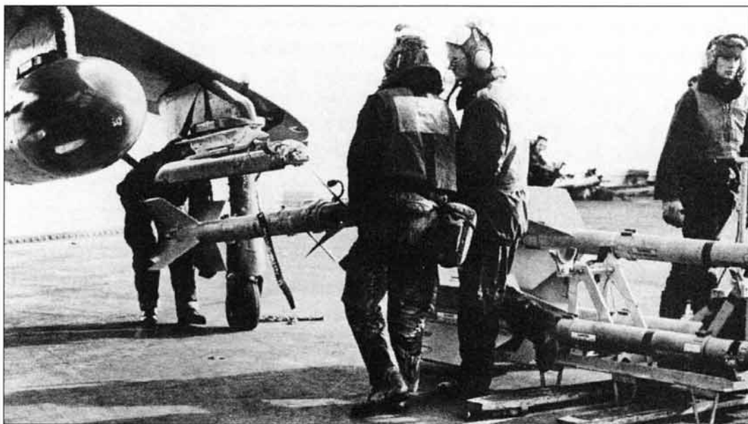
Armourers of No. 800 Squadron on board HMS Hermes prepare to load an AIM-9L Sidewinder short-range air-to-air missile onto the port underwing hardpoint of a Sea Harrier FRS Mk 1
