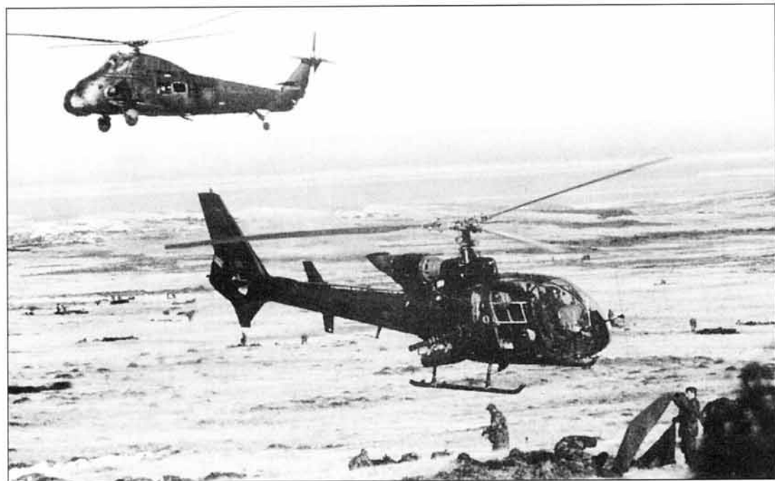
With a Wessex helicopter hovering in the background, this is a Gazelle AH.Mk 1 of No. 656 Squadron over East Falkland with multi-tube launchers for 68-mm (2.68-in) SNEB air-to-surface unguided rockets
