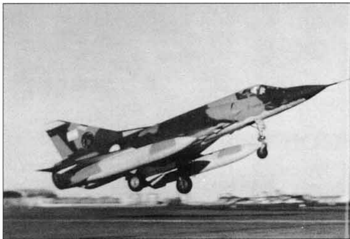
This Mirage IIIIEA of Grupo 8 is taking off on a combat air patrol with a single R530E medium-range air-to-air missile. Using semi-active radar guidance, this weapon proved far less capable than the IR-homing and therefore fully autonomous AIM-9 Sidewinder used by the British, and only one such missile was fired during the Falklands war, achieving no success as no adequate radar lock had been secured before missile launch
