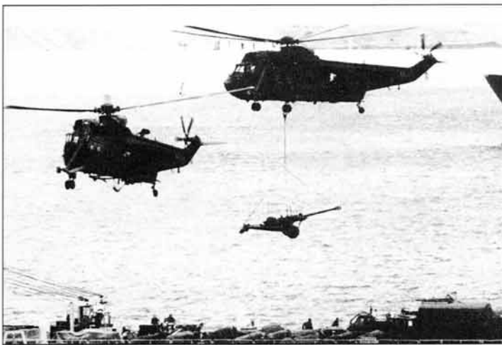
The Sea King HC.Mk 4 is the Royal Navy's counterpart of the Commando, the land-based development of the Sea King for the export market, and is used for support of the Royal Marines. This machine is pictured while lifting a 105-mm (4.13-in) L118A1 Light Gun for delivery to the troops on East Falkland
