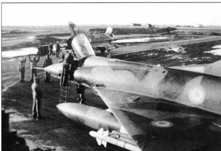
The FAA ordered a total of 17 Mirage IIIEA fighters from Dassault. The first batch of 10 aircraft was ordered in 1970, together with two Mirage IIIDA two-seaters, and seven more machines were ordered in 1977. As seen here on two aircraft of Grupo 8, the machines of the second batch were each equipped for the underwing carriage of two R550 Magic short-range air-to-air missiles. In the background is an A-4B Skyhawk of Grupo 5
