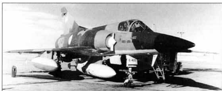
C-403 was the third Dagger received from Israel, and is seen here ready for take-off from San Julian with two 500-lb (227-kg) Mk 82 bombs and three drop tanks
