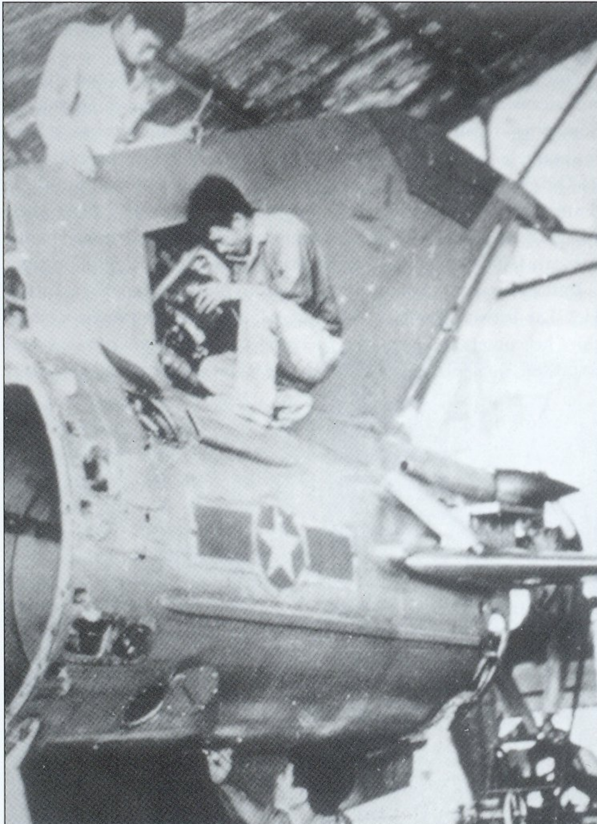
Groundcrewmembers overhaul the hydraulic system fitted in the detachable tail section of a MiG-21MF 'Fishbed-J' (VPAF Museum)
