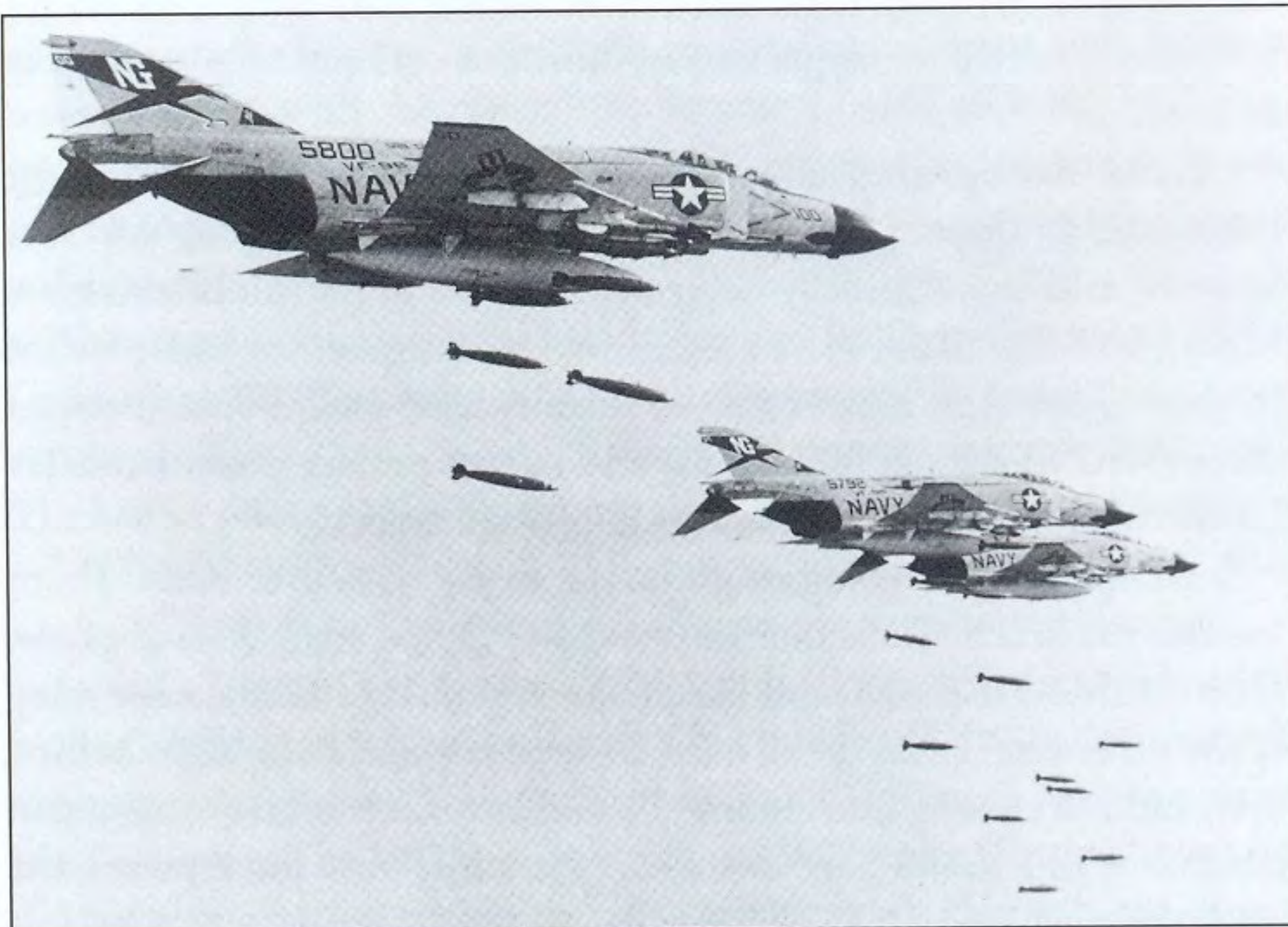
A three-ship formation of F-4Js from the 'Black Falcons' release their Mk 82 bombs (six apiece) over North Vietnam in the spring of 1972. Closest to the camera is CAG jet BuNo 155800 – a future triple MiG killer (via Peter E Davies)
