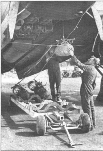
Armourers load four 250-lb bombs into the cavernous bomb-bay of a Lancaster, fitting them in front of a 4000-lb 'Cookie'. The Lancaster's huge, unobstructed bomb-bay allowed it to carry the widest possible range of weapons, making it more useful than aircraft such as the Stirling, whose bomb-bay was highly compartmentalised (Aerospace Publishing)
