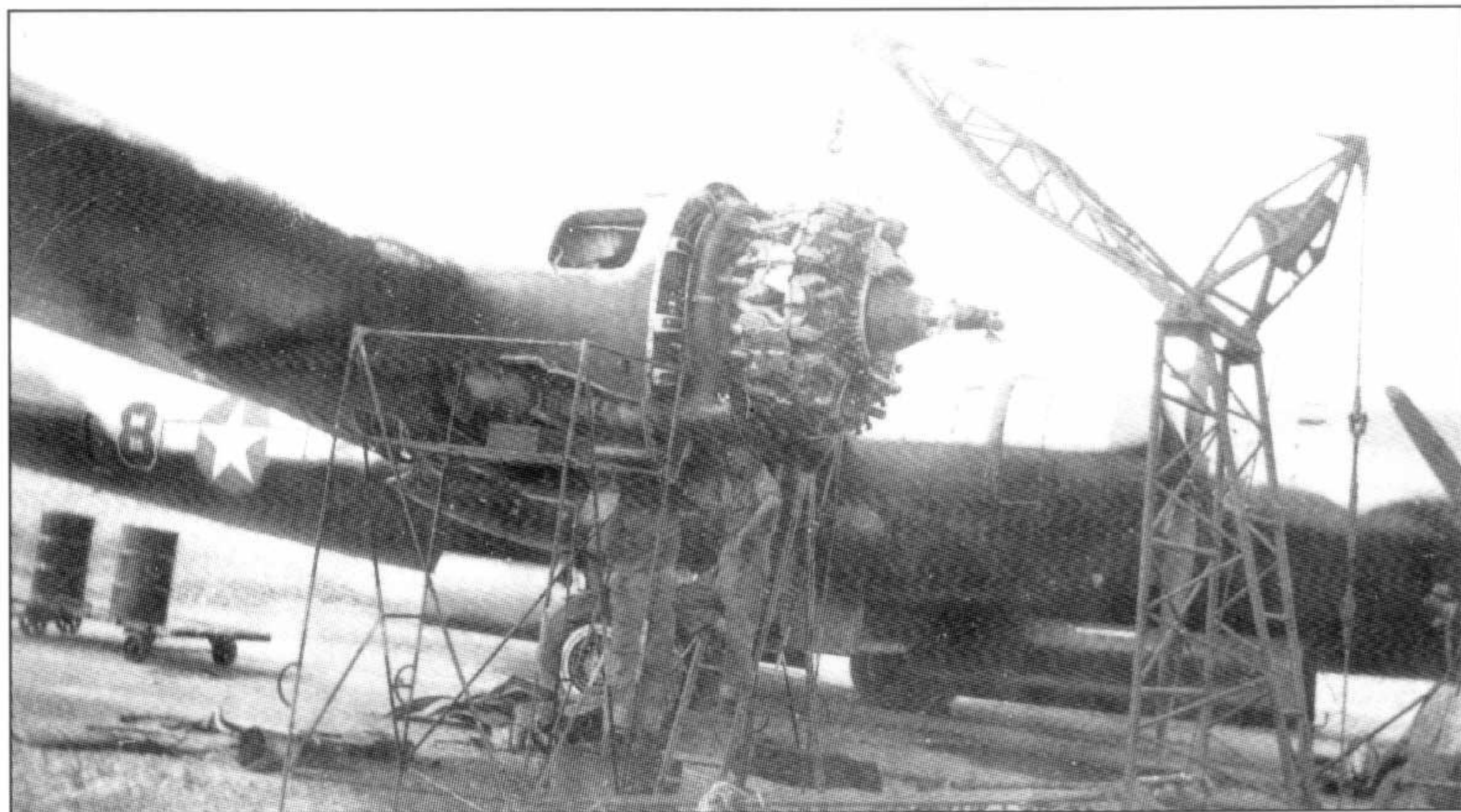
An engine change takes place in the open on a 502nd BG/315th BW Superfortress at Northwest Field, on Guam. Black undersides for night operation came along late in the war, and only a few B-29s were camouflaged. (Earl Leonard)
