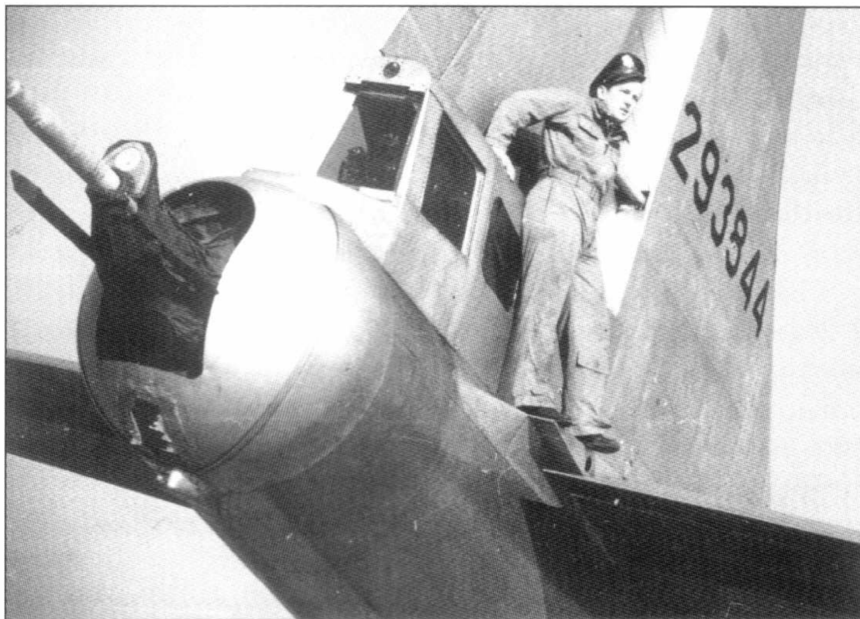
Preparing to ship to the Pacific, pilot/engineer 1Lt George Wale poses in his overalls and service hat on the horizontal stabiliser of B-29 42-93844 ANNA BELLE of the 40th BS/6th BG during a training deployment to Puerto Rico in October 1944. This view illustrates the spacious tail gunner’s position, as well as the remote-controlled 20 mm cannon, straddled by two 0.50-cal (12.7 mm) machine guns. (George Wale)
