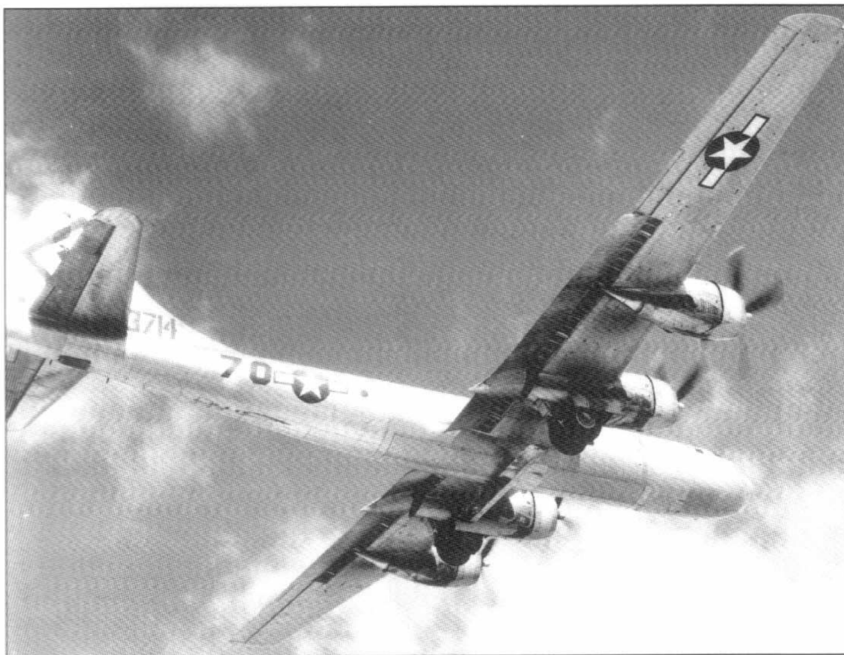
Manufactured by Bell in Atlanta, B-29B-BA 42-63714 served with the 501st BG/315th BW. Photographed climbing out from Guam’s Northwest Field, this underside view of the bomber reveals the antenna for the AN/APQ-13 Eagle ground-scanning radar, mounted beneath the fuselage at the wing juncture. This system made its combat debut with the 315th BW in the Pacific theatre late in the war. (via Frank MacSorley)
