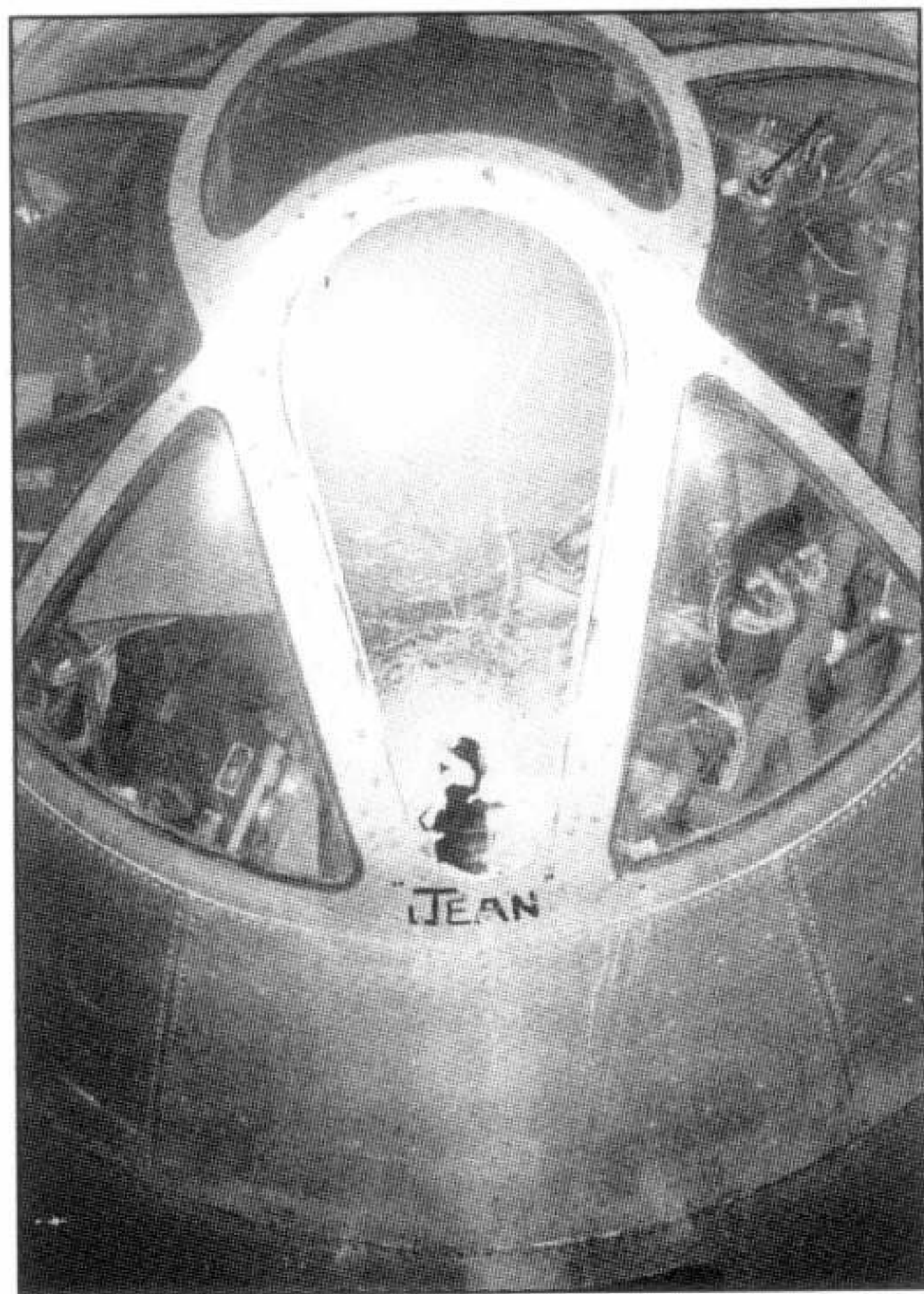
Flak struck the nose plate of this B-29, blowing a hole in the Plexiglas immediately in front of the aircraft's Norden bombsight. The name "JEAN" no doubt referred to the bomb aimer's sweetheart. (via Bill Hess)
