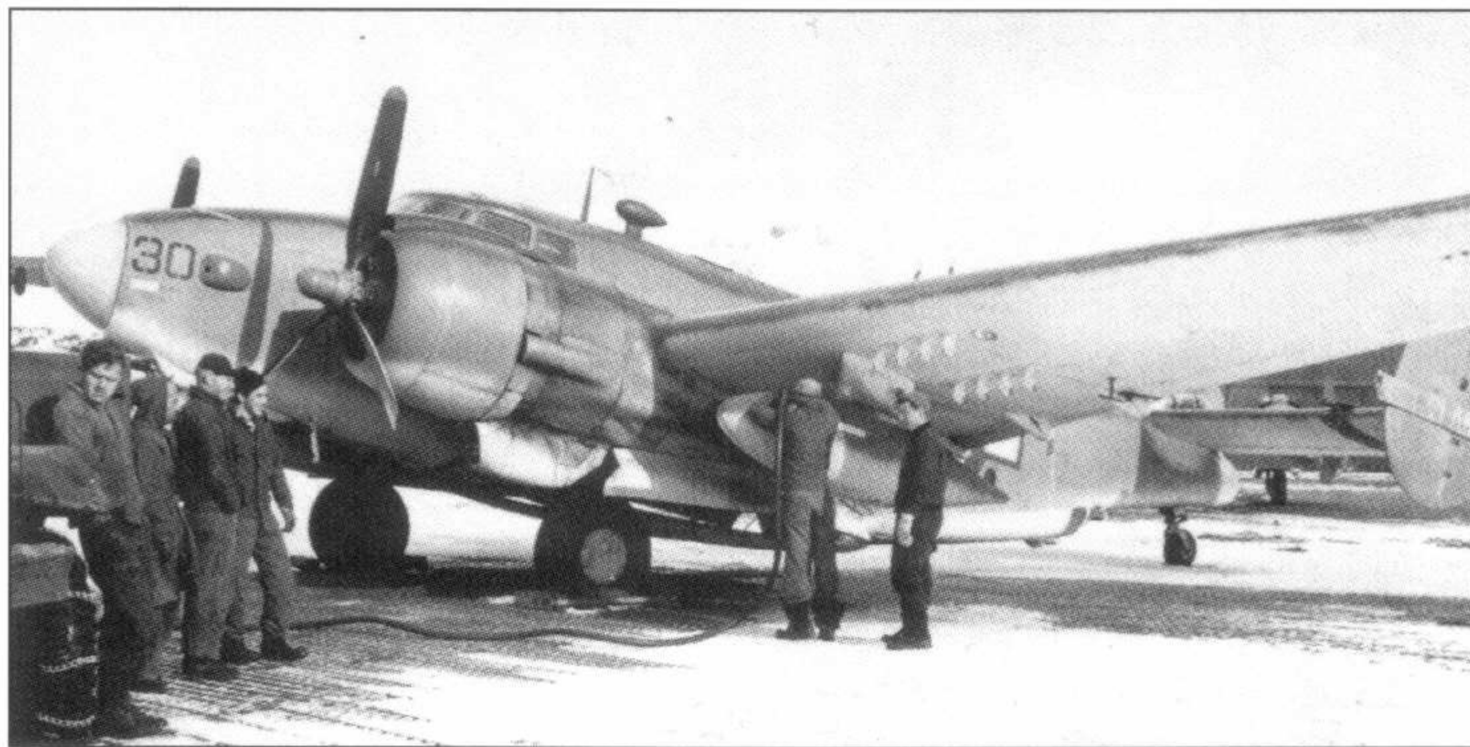
A PV-2 from VPB-139 is refuelled at Attu before conducting a strike on the Kurile Islands in April 1945. Note the mounting brackets for the underwing 5-in HVARs above the heads of the refuelling crew (via George Villasenor)
