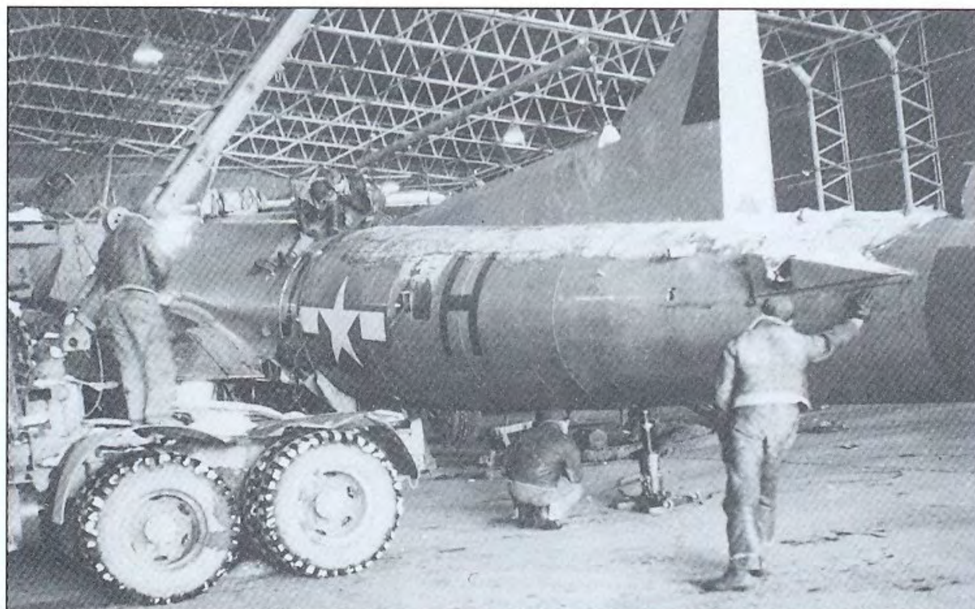
B-17G-55-DL 44-6513 Boise Belle of the 560th BS/493rd BG was photographed undergoing major repairs at Debach. Indeed, the bomber had suffered such severe battle damage that the front half of the aircraft was mated with the rear half of another damaged B-17. Boise Belle and Lt John E Silverman's crew failed to return from the Munich raid of 9 April 1945, the bomber having fallen victim to flak. All ten crewmen perished (via Truett Woodall)
